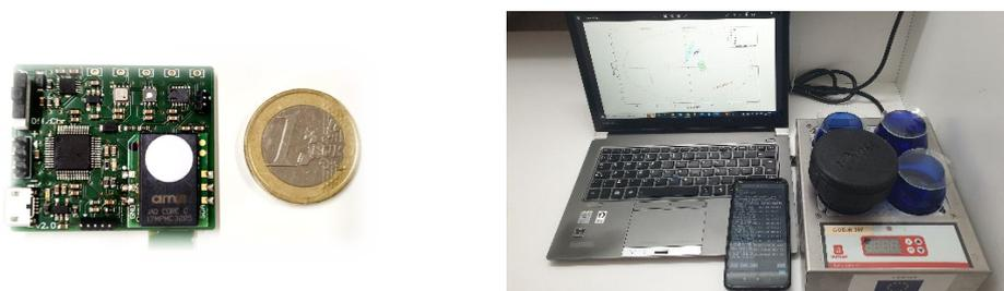
**Figure 2.** Electronic nose device (left) and the components involved in E-nose measurements (right).
