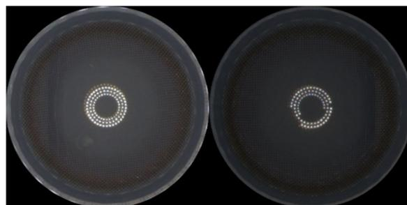
**Figure 7.** Differences in image brightness caused by external factors such as site lighting, camera lighting, and foreign substances on the camera.
