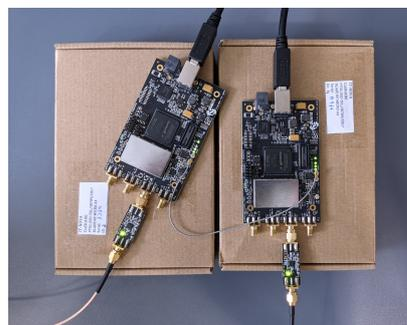
**Figure 1.** Details of the two bladeRF 2.0 micro xA4 boards with their clocks connected.
