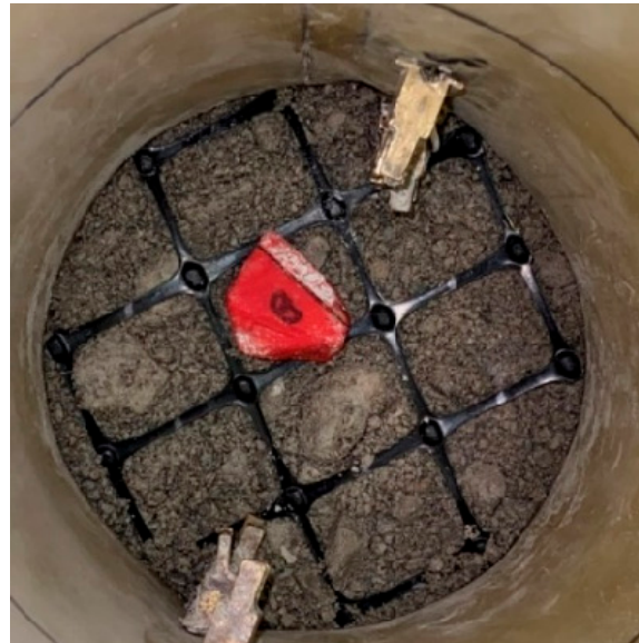
Figure 5. Geogrid and Smart Pebble placed at the TX-12 specimen’s mid-height.
