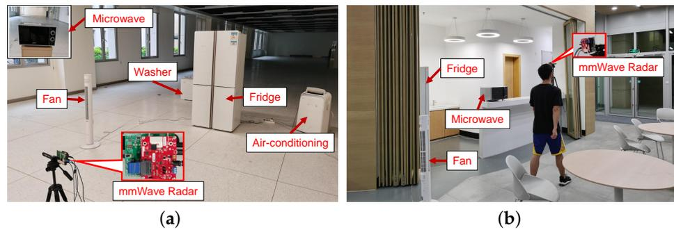
**Figure 11.** Hardware and experimental scenarios. (a) Office room; (b) Real-world scenario.
