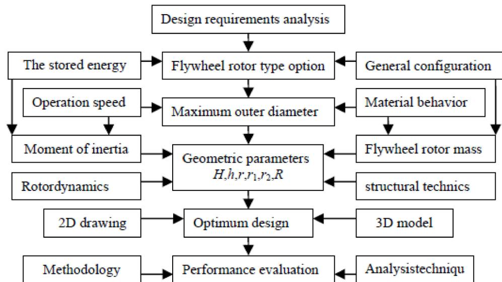
Figure 24. Flywheel rotor design process and its influence factor, reproduced with permission from [143].
