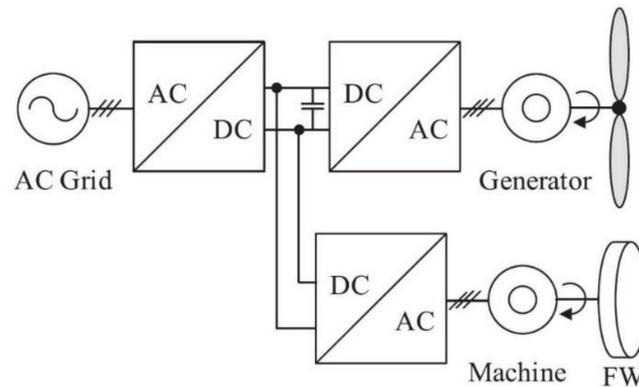
Figure 14. Back to back layout, adapted from [128].
