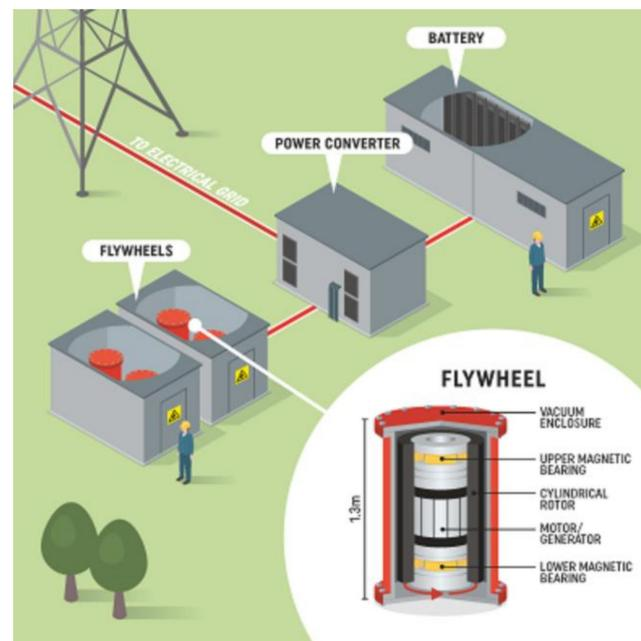
Figure 22. Domestic application of flywheel, adapted from [139].
