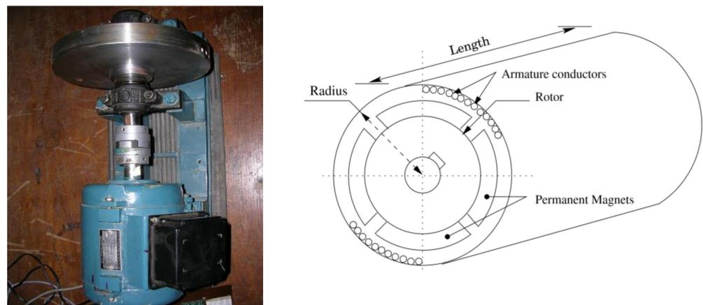
Figure 6. Brushless DC machine with flywheel adapted from [78].
