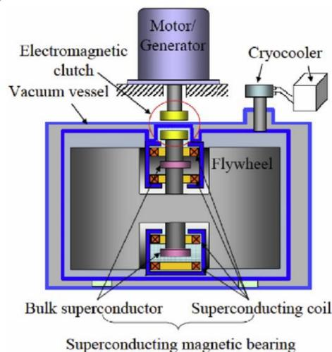
Figure 12. Superconducting magnetic bearing, adapted from [113].
