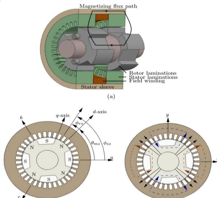
Figure 8. AC homopolar motor, adapted from [94].
