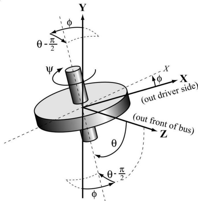
**Figure 28.** Mathematical model and coordinate systems used to analyze flywheel gyroynamics, adapted from [159].
