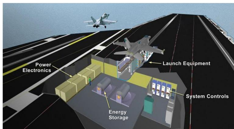
Figure 20. Electromagnetic aircraft launch system, adapted from [133].
