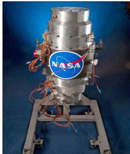
**Figure 21.** NASA flywheel and mounting bracket, adapted from [138].
