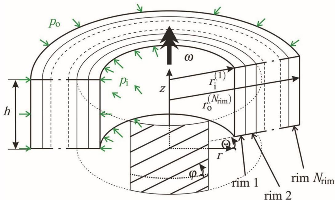
Figure 26. Rotor set up for flywheel, adapted from [146].
