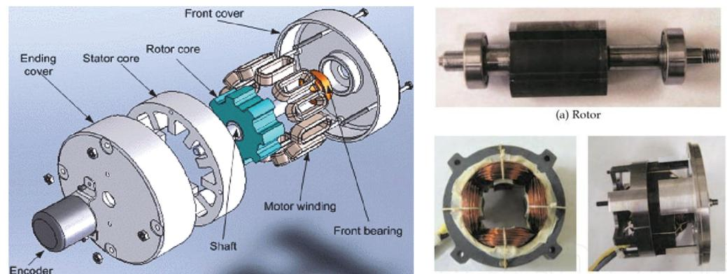
Figure 7. Switched reluctance motor for flywheel adapted from [85].
