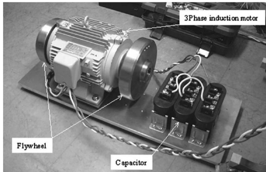
Figure 5. Flywheel energy storage system with an induction motor adapted from [73].
