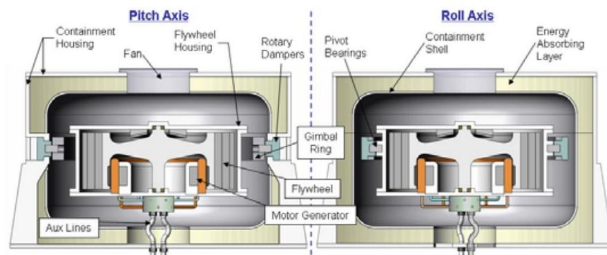
Figure 13. Flywheel containment structure, adapted from [126].
