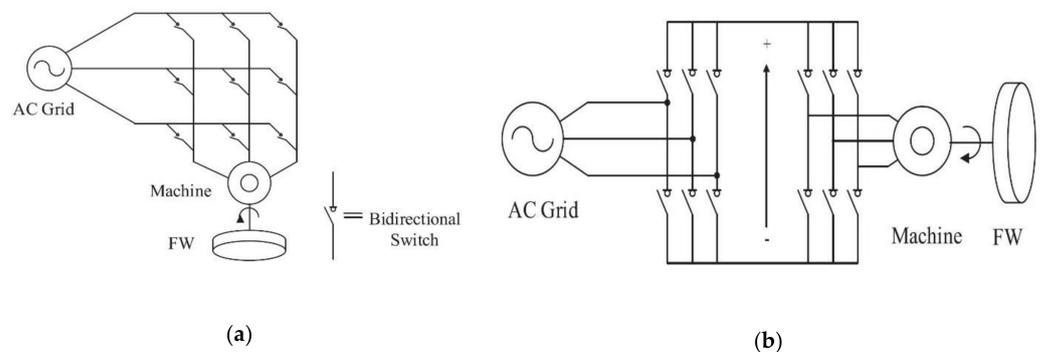
Figure 15. (a) Direct matrix converter, (b) indirect matrix converter, reproduced with permission from [48].
