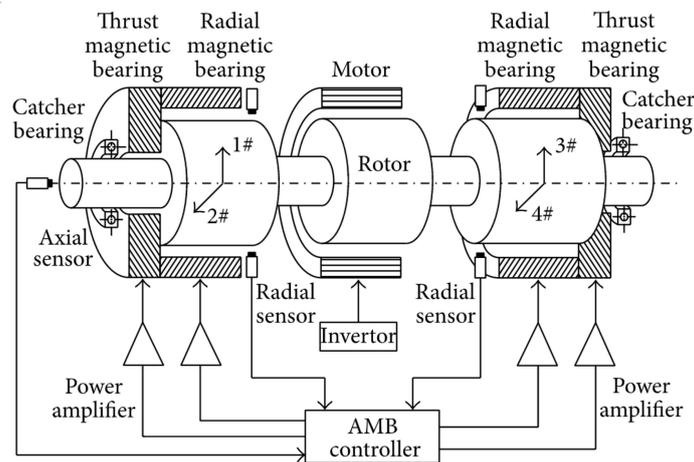
Figure 11. Active magnetic bearing system, adapted from [110].
