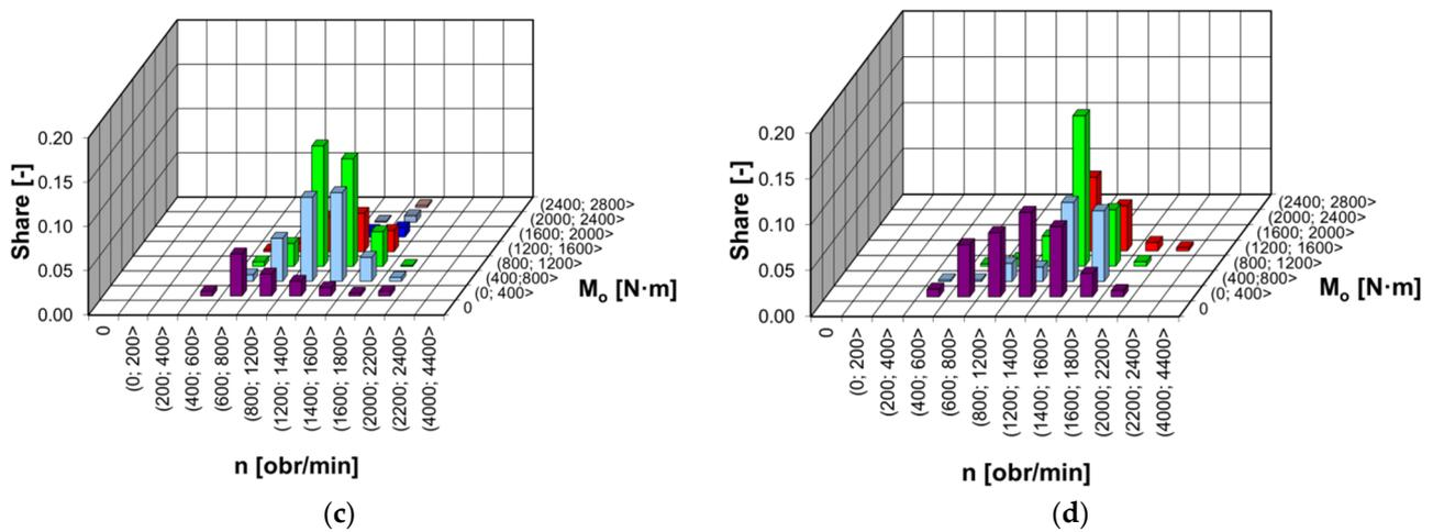
Figure 7. Operating time share as a function of engine load and engine speed during individual test stage, (a) stage one, (b) stage two, (c) stage three, (d) stage four—bitumen-paved road.
