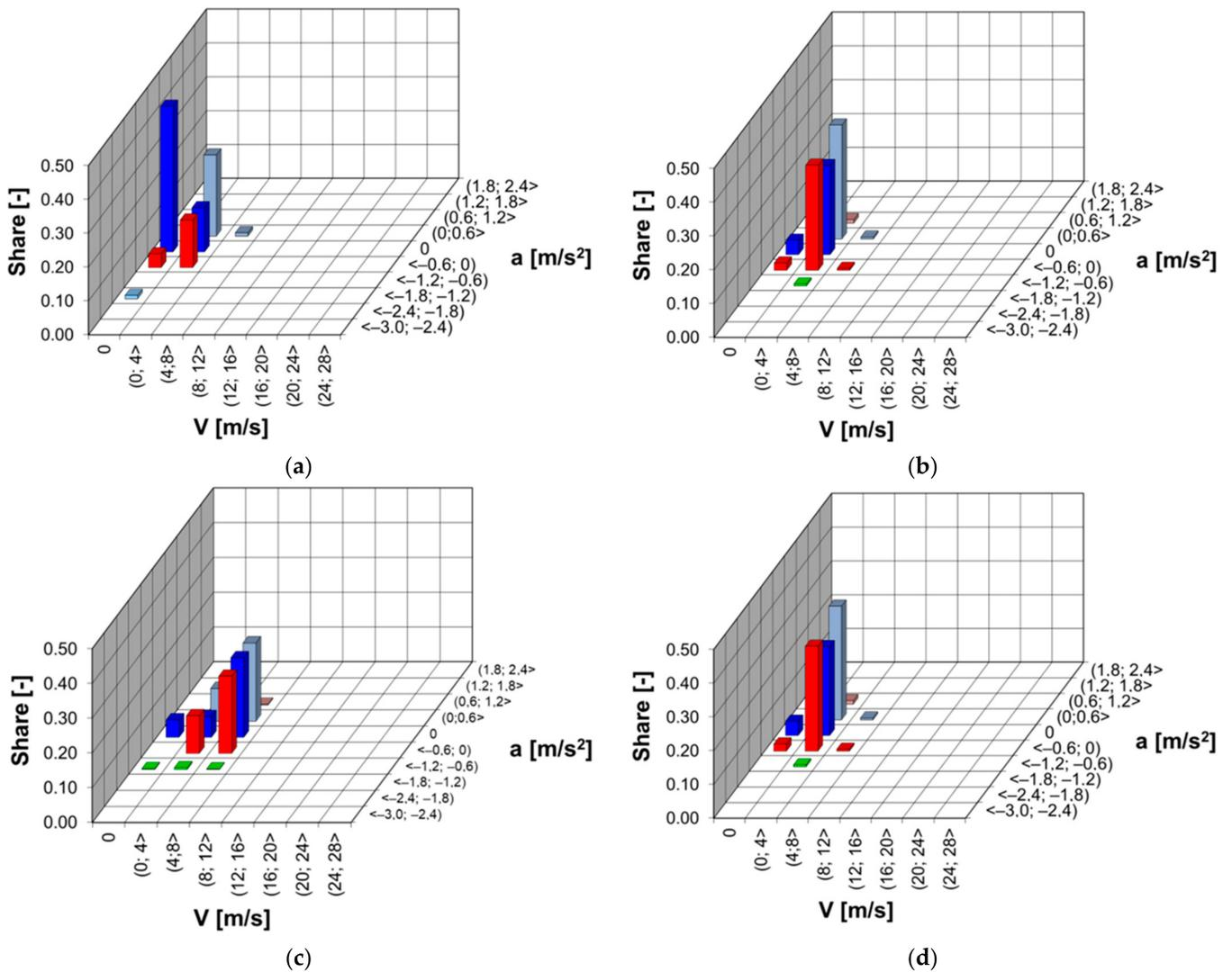
Figure 6. Operating time share as a function of speed and acceleration during individual test stages, (a) stage one, (b) stage two, (c) stage three, (d) stage four—bitumen-paved road.
