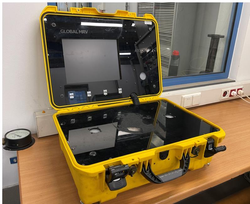
Figure 2. Portable emission measurement system Axion RS+.
