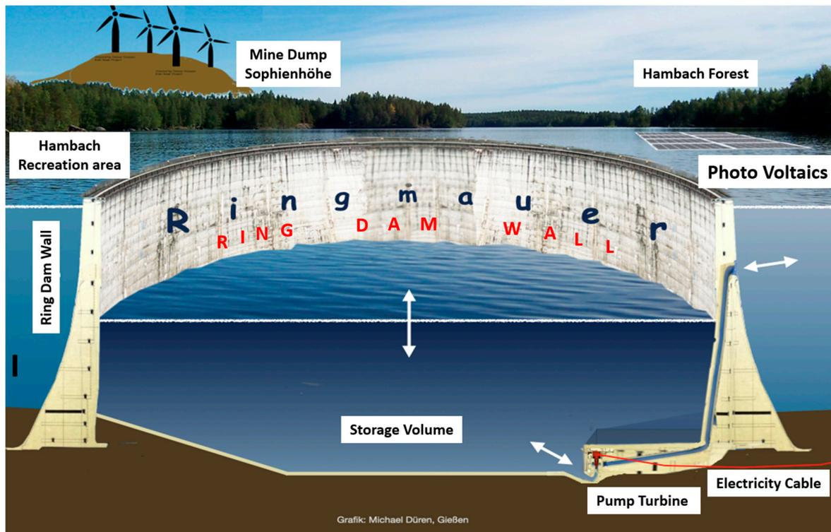
**Figure 13.** Ring dam wall (“Ringmauer-Staubecken”): the lower basin (“storage volume”) of a huge PSH using the surrounding lake as the upper basin [10,47].
