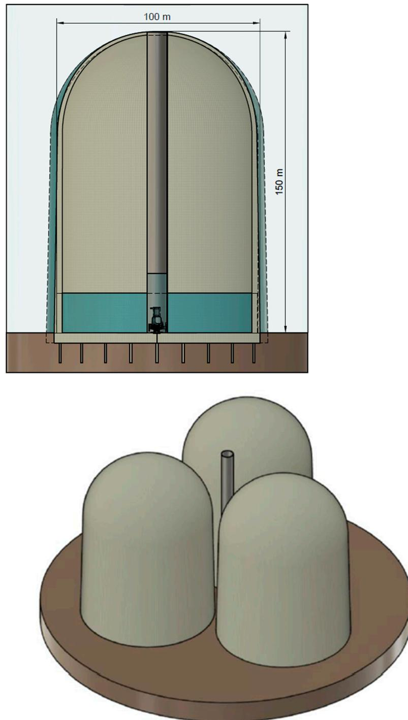
**Figure 12.** Upper part: Cross section of a bell-shaped storage tank, Lower part: Cloverleaf storage system.
