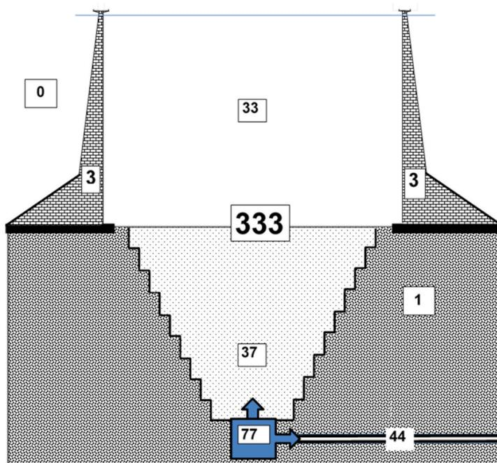
**Figure 14.** Lower storage basin 333, consisting of ring dam wall 3 and bottom storage hole 37, of a PSH operating in residual lake 0 of a former open cast mine. Storage hole 37 will be dredged out of the later lakebed 1 with the existing open cast mining machines (for more detail, see [10,47]).
