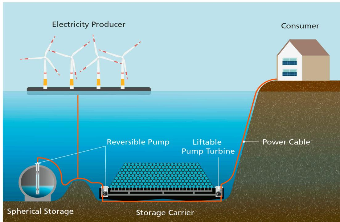
**Figure 5.** Scheme of the U.PSH energy storage system.
