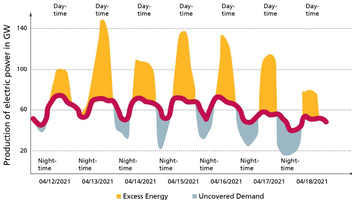
**Figure 1.** Electric energy production of the week from 12 to 18 April 2021 by wind power and photovoltaics in Germany scaled with factor 4.5 [9] (see text).
