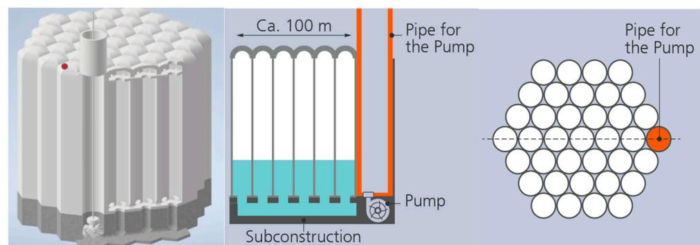
**Figure 11.** Sketch of segment A. **Left:** the view from outside, middle: sectional view. The outer pipes have thicker walls to resist the high water pressure; the inner pipes form one storage volume and thus always have the same low pressure. At the bottom of one pipe (here, the one on the right), the turbine is mounted. This pipe provides the water in- and outlet. The wall of this pipe is thicker and prepared to resist the high inner water pressure. **Right:** Top view of segment A.
