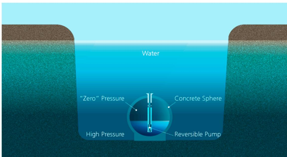
**Figure 4.** Schematic display of the “sphere” U.PSH energy storage system. Notice: the reversible hydroelectric turbine should be mounted at the deepest point of the sphere.
