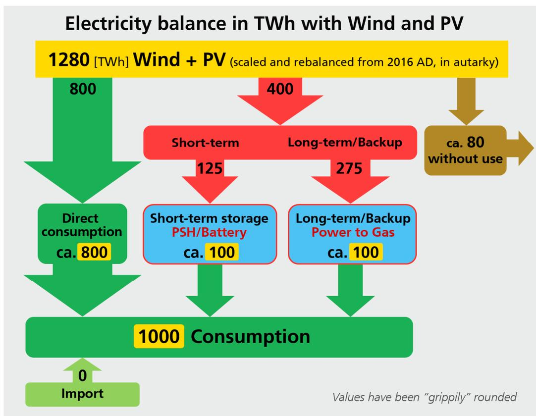
**Figure 3.** Typical yearly overall electricity flux scheme in Germany when the energy transition is completed and no imports are needed, ensuring autarky [10].
