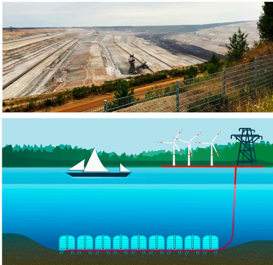
**Figure 10.** Upper part: View of the present lignite mine of Hambach/Germany (Photo H. Schmidt-Böcking), Lower part: Future vision of U.PSH in the flooded lake as recreation park for sailing.
