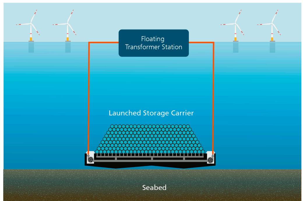
**Figure 9.** Floating wind turbines with energy storage U.PSH on the ocean floor.
