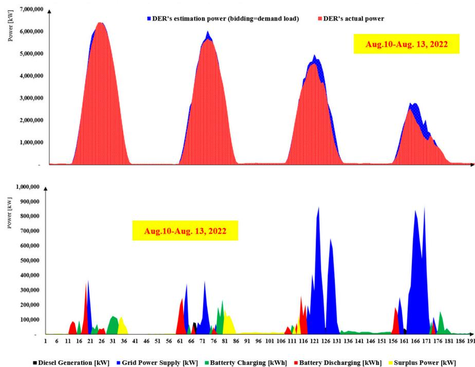
**Figure 4.** The upper half of the graph represents the demand load and actual renewable energy generation data. The lower half of the graph indicates power supply by the DG, grid, and surplus power, as well as battery charge and discharge.
