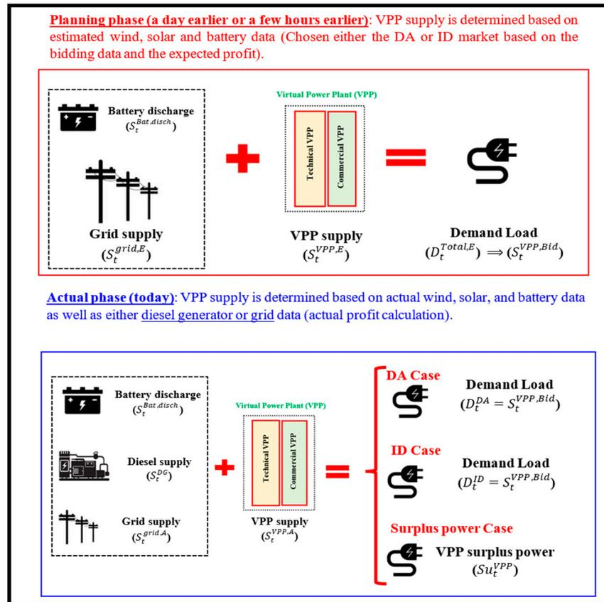
Figure 2. Planning and actual phases of the VPP model.
