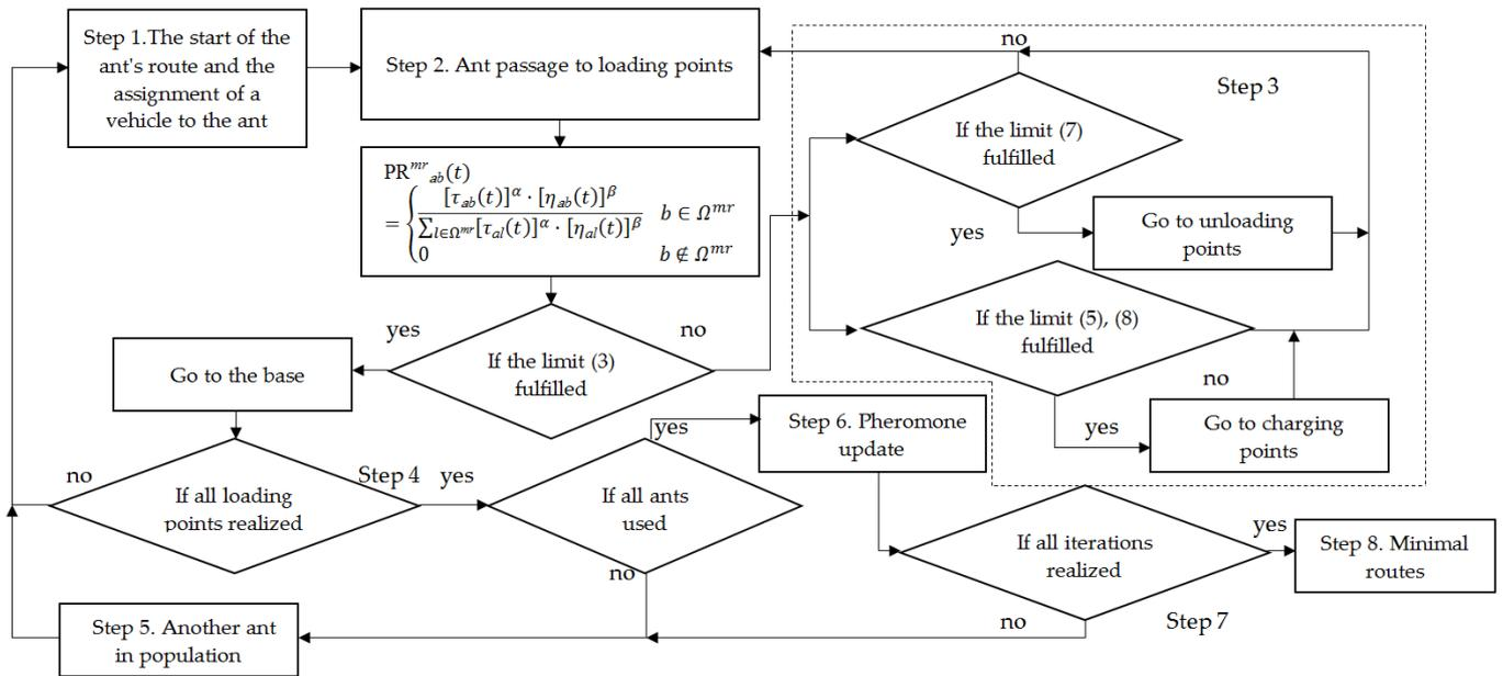
Figure 3. Diagram of the ant algorithm’s operation.
