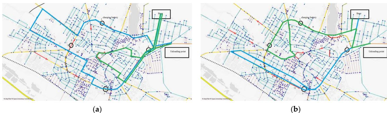
Figure 8. The driving route of the vehicles created by the ant algorithm: (a) the first vehicle; (b) the second vehicle.
