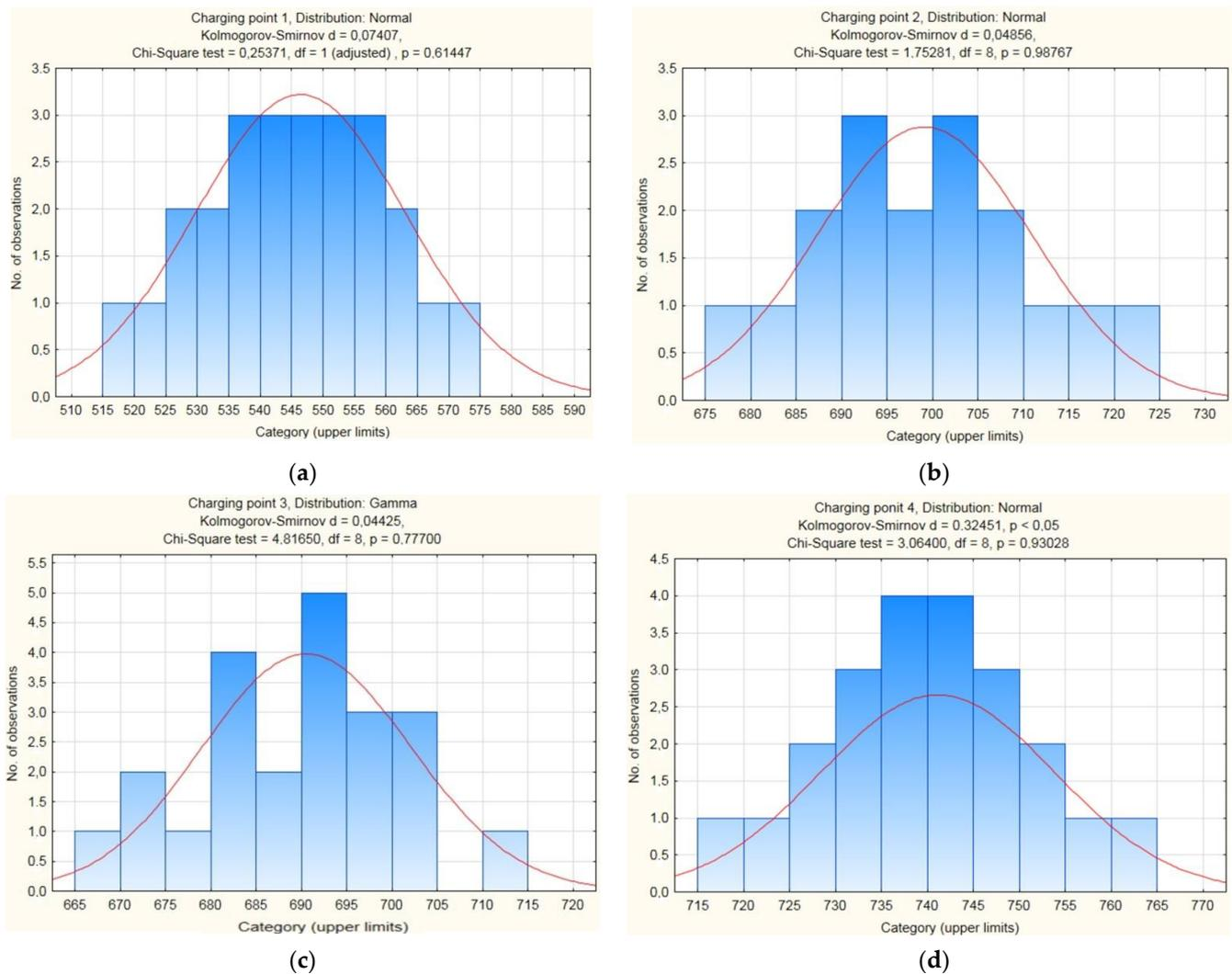
**Figure 6.** Theoretical distributions of the uncertainty of charging point operation, (a) point 1, (b) point 2, (c) point 3, and (d) point 4.
