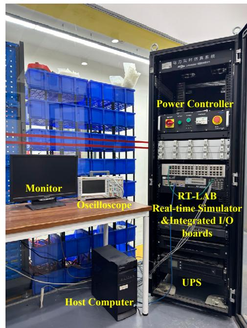
Figure 12. Hardware-in-the-loop experimental platform.
