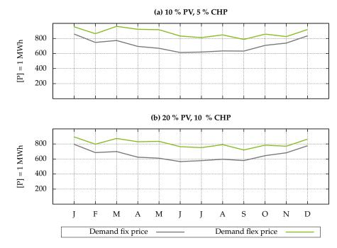
**Figure 11.** Total demand per month for regional green electricity in fixed and flex price systems over one year for PV and CHP expansion stages (a) 10% PV, 5% CHP and (b) 20% PV, 10% CHP.
