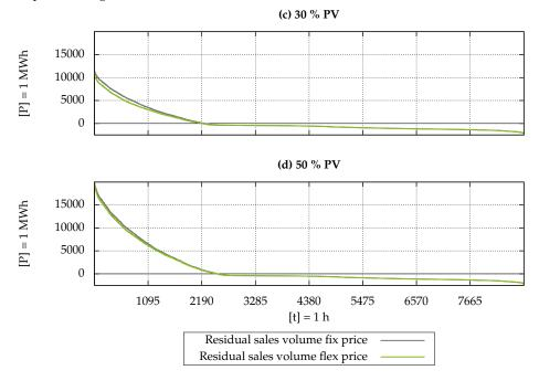
**Figure 9.** Ordered residual sales volume in fixed and flex price scenarios over one year for PV expansion stages (c) 30% PV and (d) 50% PV.
