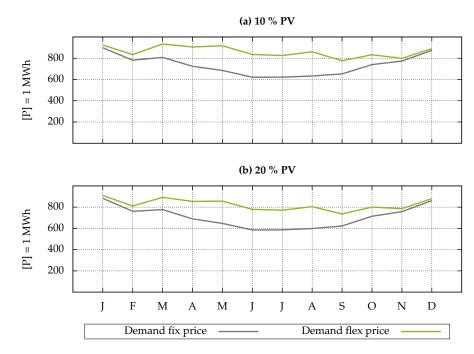
**Figure 4.** Total demand per month for regional green electricity in fixed and flex price systems over one year for PV expansion stages (a) 10% PV and (b) 20% PV.
