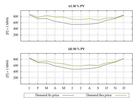
**Figure 5.** Total demand per month for regional green electricity in fixed and flex price systems over one year for PV expansion stages (c) 30% PV and (d) 50% PV.
