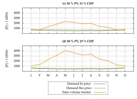
**Figure 14.** Relation between total demand in fixed and flex price scenarios and total sales volume per month for regional green electricity over one year for PV and CHP expansion stages (c) 30% PV, 15% CHP and (d) 50% PV, 25% CHP.
