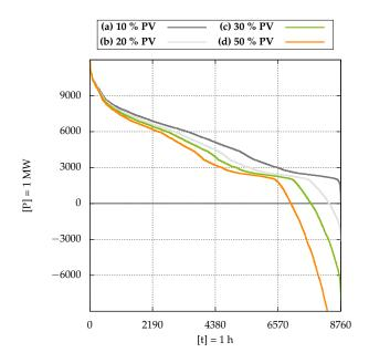
**Figure 3.** Ordered residual load profile (region) of the supply system over one year for different PV expansion stages (a)–(d).
