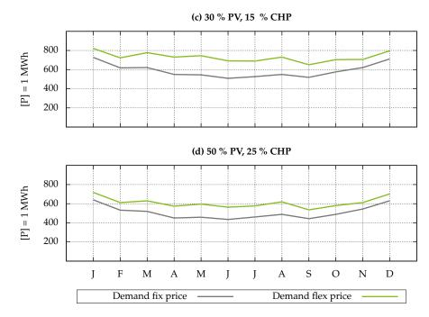
**Figure 12.** Total demand per month for regional green electricity in fixed and flex price systems over one year for PV and CHP expansion stages (c) 30% PV, 15% CHP and (d) 50% PV, 25% CHP.
