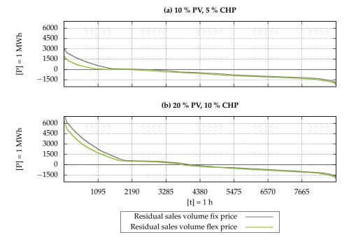
**Figure 15.** Ordered residual sales volume in fixed and flex price scenarios over one year for PV and CHP expansion stages (a) 10% PV, 5% CHP and (b) 20% PV, 10% CHP.
