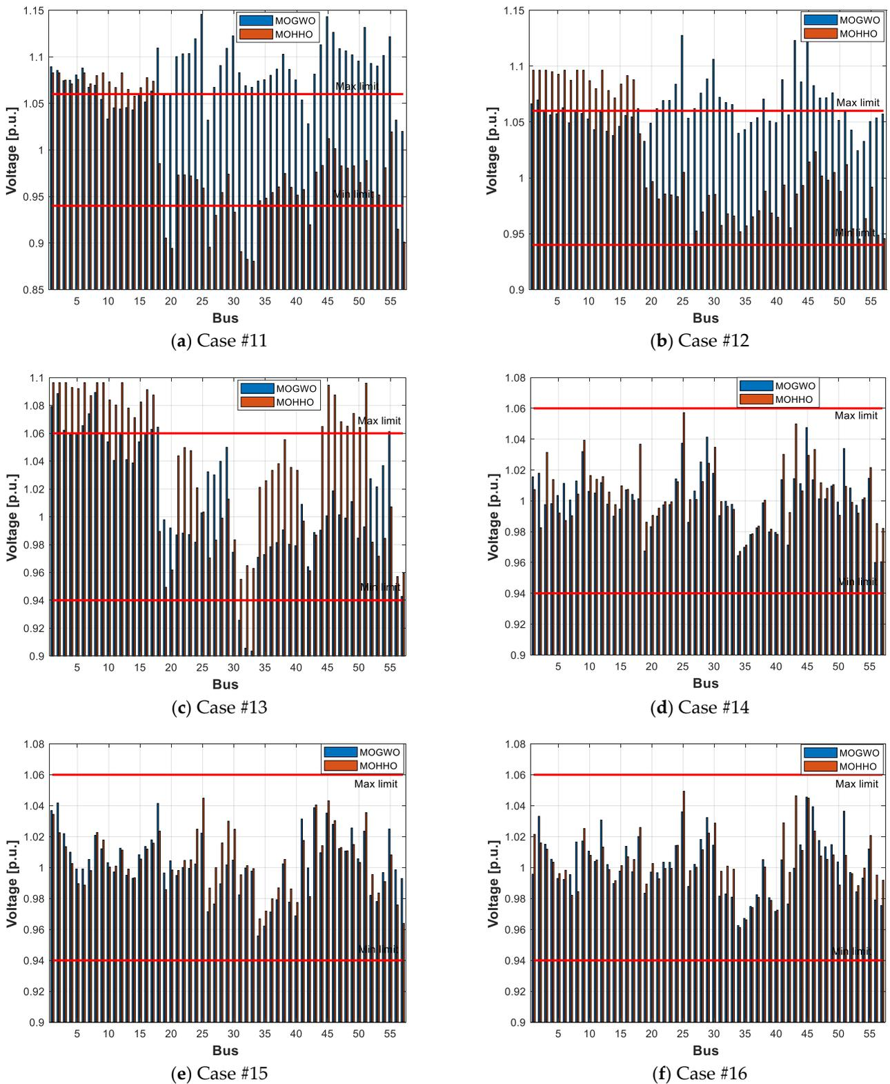
Figure 13. The voltage profiles for Cases (11–16).
