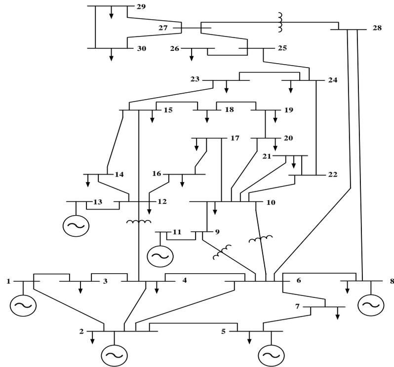
Figure A1. The single line diagram of IEEE 30 bus system.
