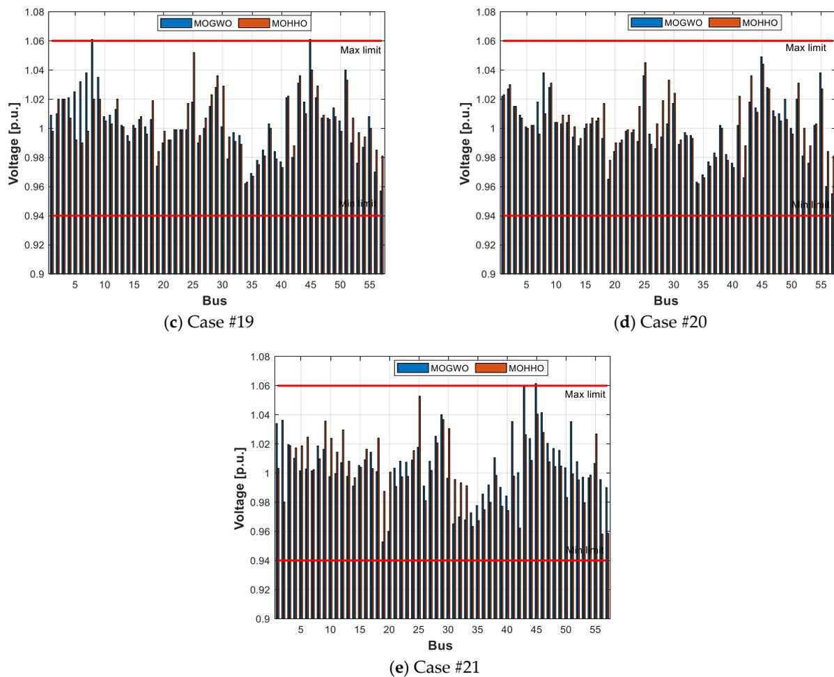
**Figure 15.** The voltage profiles for Cases (17–21).
