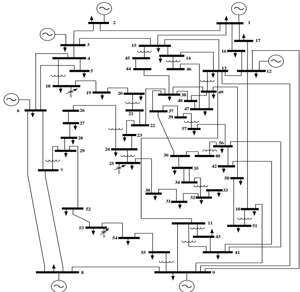
Figure A2. The single line diagram of IEEE 57 bus system.
