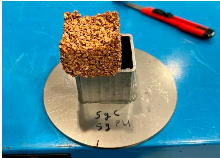
**Figure 3.** Polyurethane/cork test specimen, mixed at 1:1 ratio of 5 g cork and 5 g polyurethane, removed from mould.
