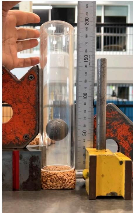
Figure 5. Energy absorption test rig and specimen showing steel ball at maximum rebound height.
