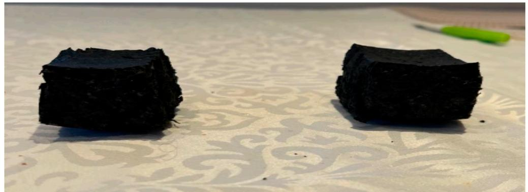
**Figure 4.** Expanded polystyrene test specimens extracted from scooter helmet.
