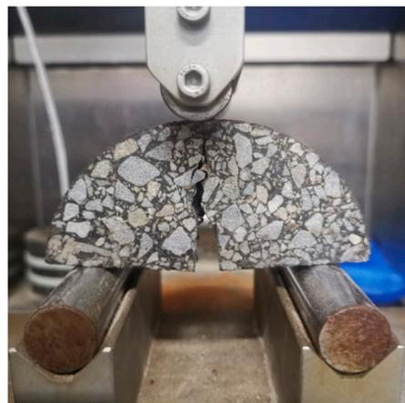
**Figure 6.** Semi-circular specimen test set.
