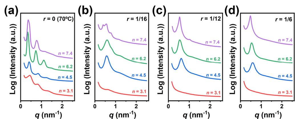
**Figure 1.** SAXS profiles of PVPS<sub>*n*</sub>-*b*-PEO<sub>210</sub>-*b*-PVPS<sub>*n*</sub>/LiTFSI blends with (a)  $r = 0$ , obtained at 70 °C, (b)  $r = 1/16$ , (c)  $r = 1/12$ , and (d)  $r = 1/6$  at 30 °C.
