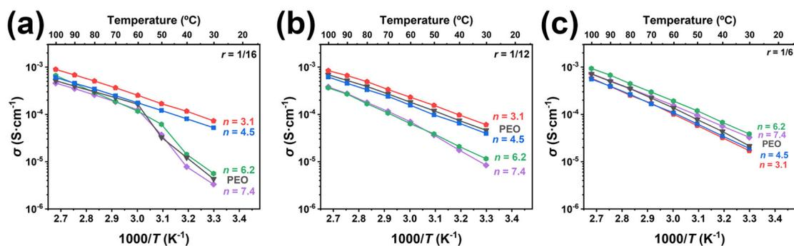
**Figure 4.** Ionic conductivities ( $\sigma$ ) of PVPS<sub>*n*</sub>-*b*-PEO<sub>210</sub>-*b*-PVPS<sub>*n*</sub>/LiTFSI and PEO<sub>210</sub>/LiTFSI hybrids at different doping ratios. (a)  $r = 1/16$ , (b)  $r = 1/12$ , and (c)  $r = 1/6$ .
