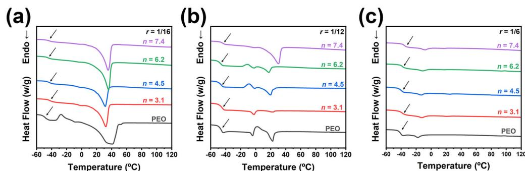
**Figure 2.** DSC 2nd heating curves of PEO<sub>210</sub>/LiTFSI and PVPS<sub>*n*</sub>-*b*-PEO<sub>210</sub>-*b*-PVPS<sub>*n*</sub>/LiTFSI with different doping ratios. (a)  $r = 1/16$ , (b)  $r = 1/12$ , and (c)  $r = 1/6$ .
