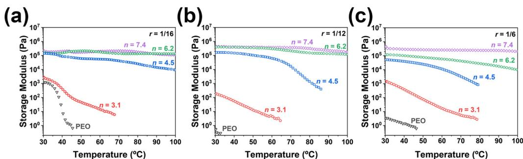
**Figure 3.** Storage moduli of PVPS<sub>*n*</sub>-*b*-PEO<sub>210</sub>-*b*-PVPS<sub>*n*</sub>/LiTFSI and PEO<sub>210</sub>/LiTFSI hybrids at different doping ratios. (a)  $r = 1/16$ , (b)  $r = 1/12$ , and (c)  $r = 1/6$ .
