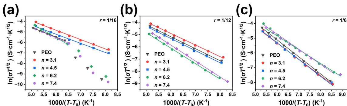
**Figure 5.** VTF plots for (a) PVPS-*b*-PEO-*b*-PVPS/LiTFSI with  $r = 1/16$ , (b) PVPS-*b*-PEO-*b*-PVPS/LiTFSI with  $r = 1/12$ , and (c) PVPS-*b*-PEO-*b*-PVPS/LiTFSI with  $r = 1/6$ .
