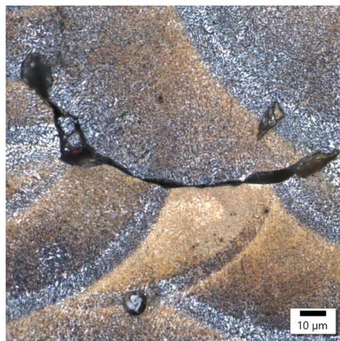
Figure 11. Sample 34 showing porosity on the boundaries of melting pools.
