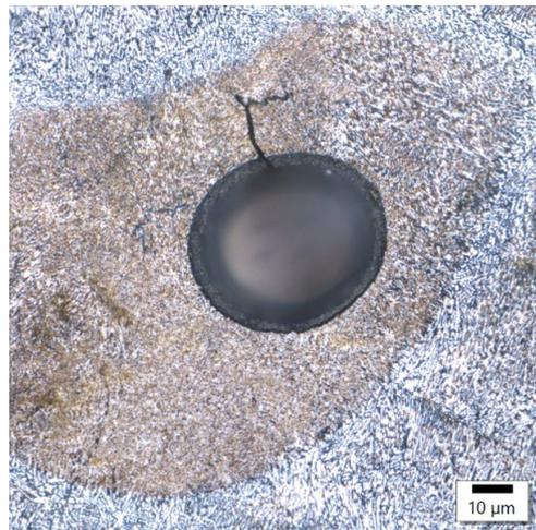
Figure 12. 3 Sample 3's spherical pore.
