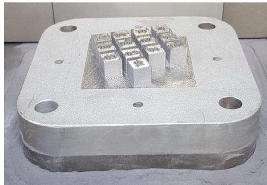
**Figure 1.** Distribution of printed samples on the substrate plate.
