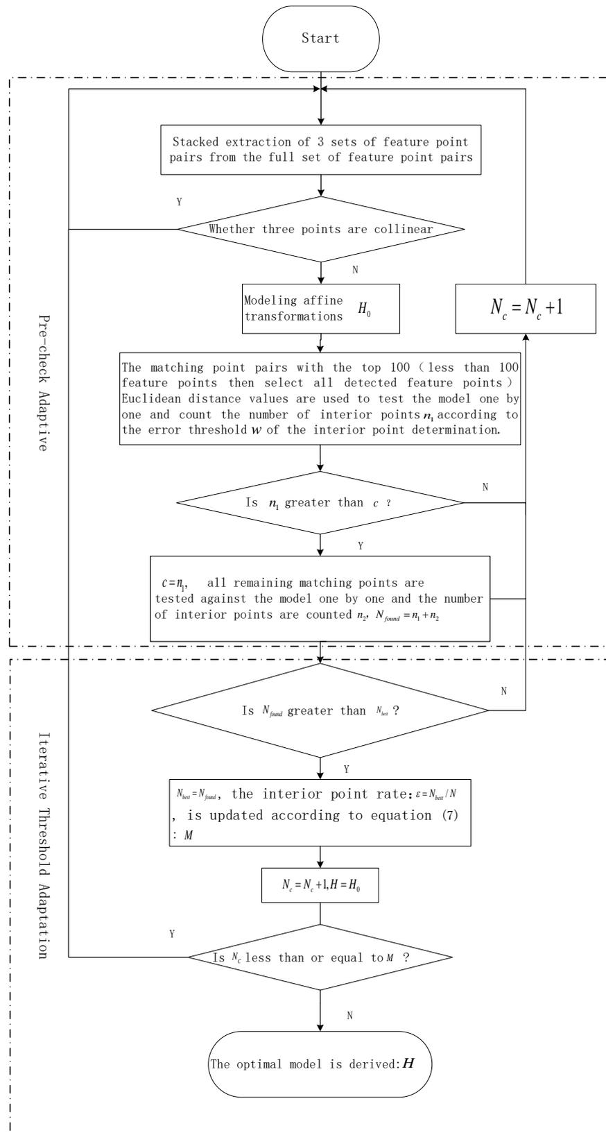
Figure 2. Schematic diagram of the adaptive RANSAC algorithm.
