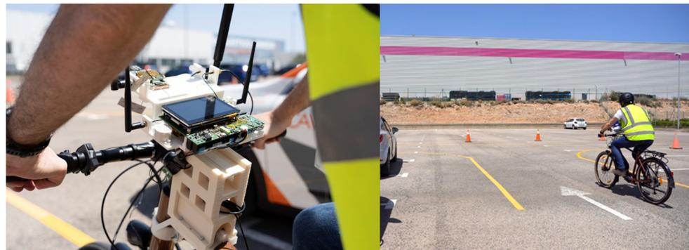
**Figure 2.** (left): OBU physical test device; (right): physical testing of V2X system in the user study.
