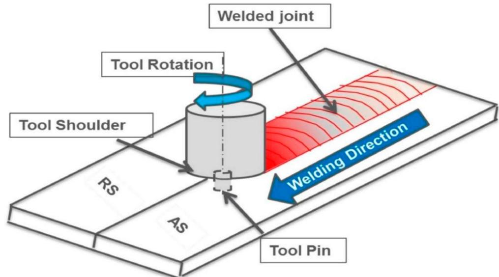
Figure 5. FSW process [27].
