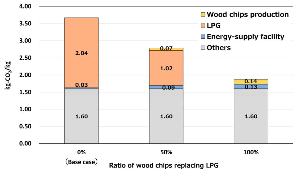
**Figure 7.** LC-CO<sub>2</sub> emissions by wood chip ratio and their breakdown.
