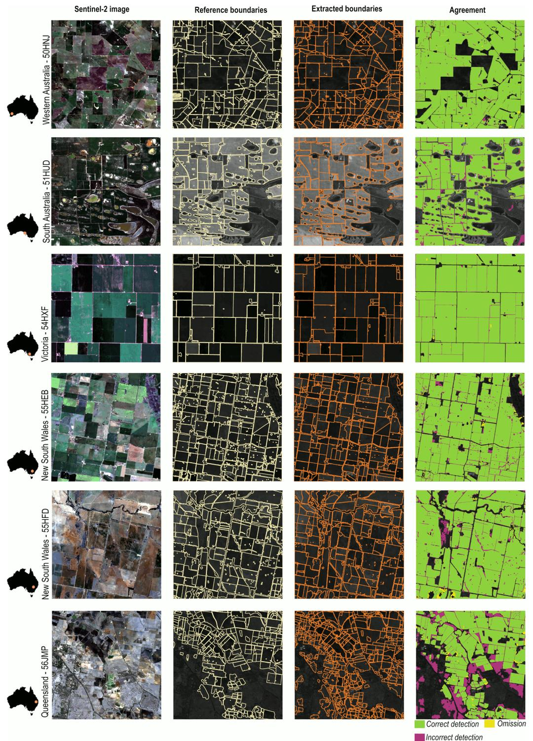
**Figure 9.** Instance segmentation outputs in a range of Australian cropping regions (5 km × 5 km). These outputs were obtained for the source-to-target case, that is, a FracTAL ResUNet model trained on South African data and applied across Australia.
