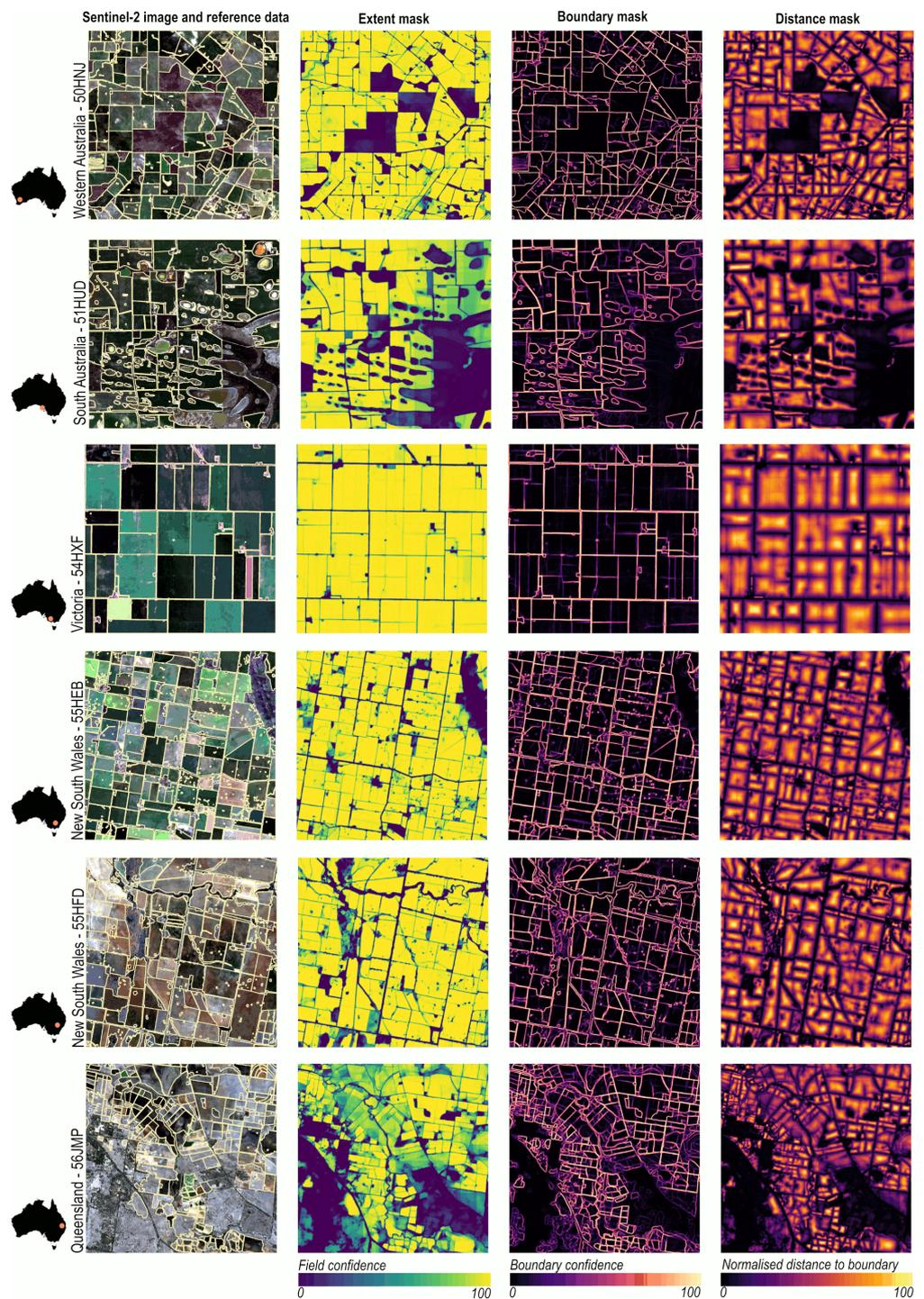
**Figure 6.** Semantic segmentation outputs in a range of Australian cropping regions (5 km × 5 km). These outputs were obtained for the source-to-target case, that is, a FracTAL ResUNet trained on South African data and applied across Australia.
