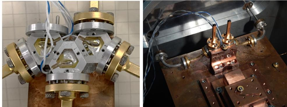
**Figure 18.** The cryogenic latching-circulator receiver protector for HUSIR (**left**) and its mounting in the 20 K dewar (**right**). The picture on the (**right**) shows mounting provisions for W-band receiver hardware, which is not installed in this picture.
