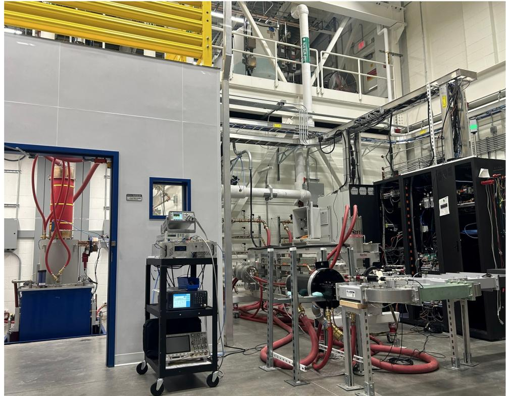
**Figure 15.** The interior of the new transmitter facility with one of two klystrons (left) and its output waveguide and isolator (right). Coolant water is provided from the mezzanine level above.
