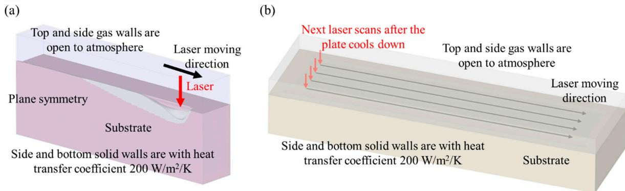
**Figure 1.** Boundary conditions: (a) single-track, (b) multiple-track.
