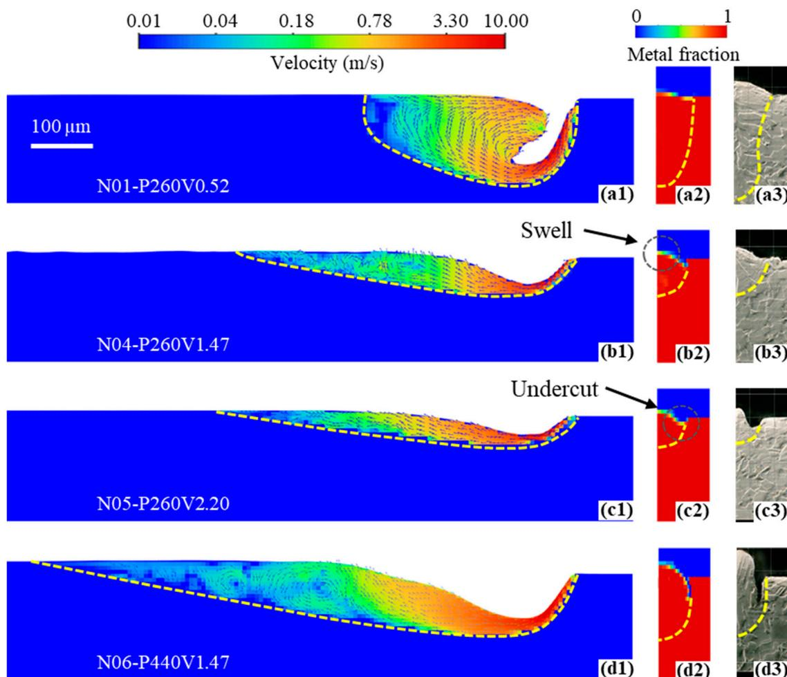
**Figure 9.** Predicted velocity and melt pool in simulations (a1–d2) and melt pool cross sections in experiments (a3–d3) under different laser powers and speeds. (a1–a3)  $P = 260$  W,  $V = 0.52$  m/s; (b1–b3)  $P = 260$  W,  $V = 1.47$  m/s; (c1–c3)  $P = 260$  W,  $V = 2.20$  m/s; (d1–d3)  $P = 440$  W,  $V = 1.47$  m/s.
