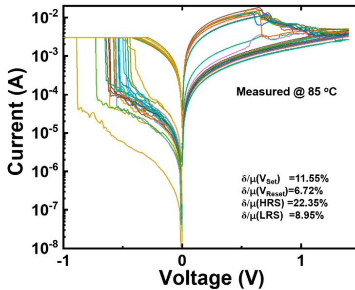
Figure 5. Typical bipolar resistor switch  $I$ - $V$  characteristic curves of the S3 device at 85 °C.
