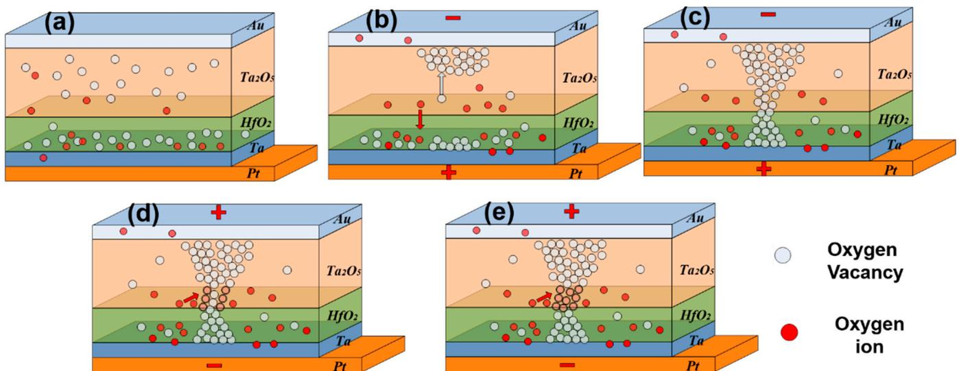
**Figure 1.** A schematic qualitative model of switching modes in the Au/ $\text{Ta}_2\text{O}_5$ / $\text{HfO}_2$ /Ta/Pt device. (a) Initial state, (b) set process, (c) LRS, (d) reset process, (e) HRS.
