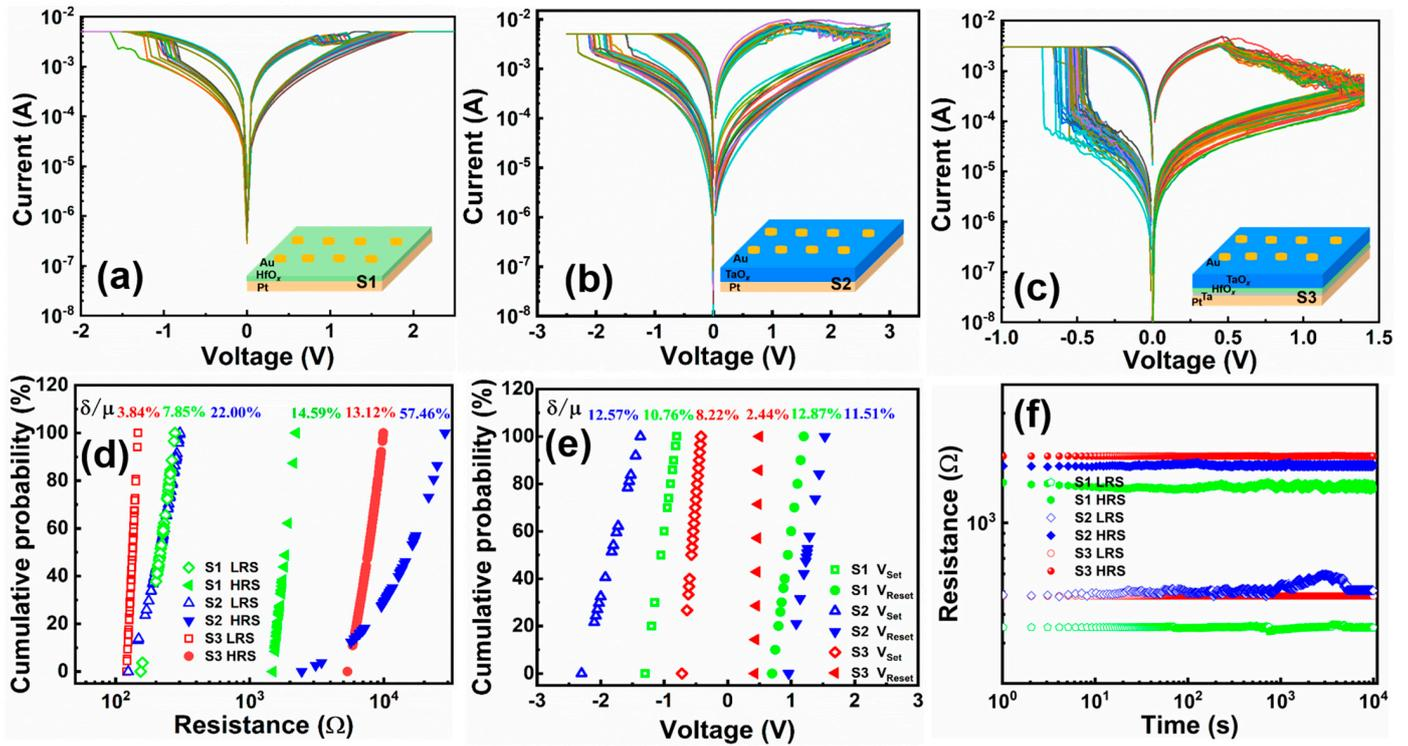
**Figure 3.** Typical bipolar resistor switch  $I-V$  characteristic curves of S1 (a), S2 (b), and S3 (c). The insets are the corresponding device structures. (d) The cumulative probability distribution of the high and low resistance values of the devices. (e) Cumulative probability distribution of switching voltages. (f) Retention testing of S1, S2, and S3. The relative fluctuations can be expressed by the equation  $\delta/\mu$  ( $\delta$  is the standard deviation and  $\mu$  is the mean).
