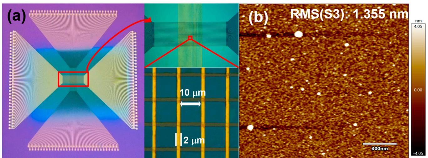
**Figure 2.** (a) Optical image and scanning electron image of the  $64 \times 64$  crossbar array, (b) AFM image of S3.
