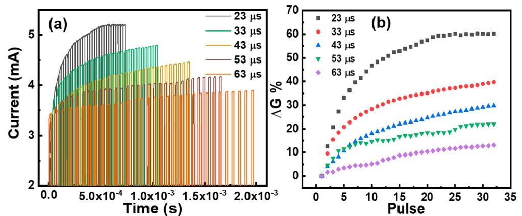
**Figure 7.** Pulse-frequency dependent characteristics of the device. (a) Voltage pulses of different periods regulate the change in the current of the S3 device. (b) Variations in the rate of change of conductance with the period of applied pulses.
