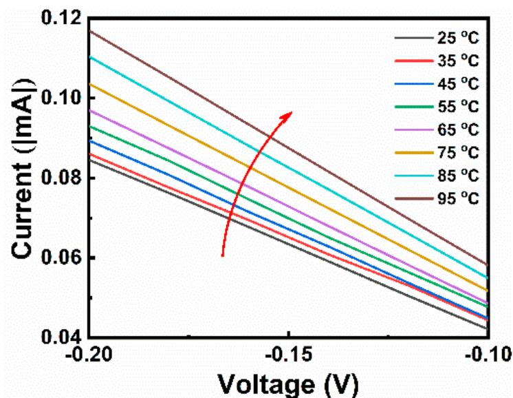
**Figure 4.** Temperature-dependent  $I$ - $V$  curves for S3 operated in LRS mode at different temperatures, ranging from 25 to 95 °C.
