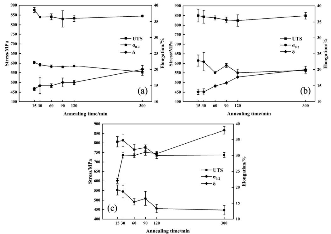
**Figure 9.** Tensile properties of Ti<sub>50</sub>Ni<sub>47</sub>Fe<sub>3</sub> alloys with different annealing processes. (a) Annealed at 400 °C; (b) annealed at 500 °C; (c) annealed at 600 °C.
