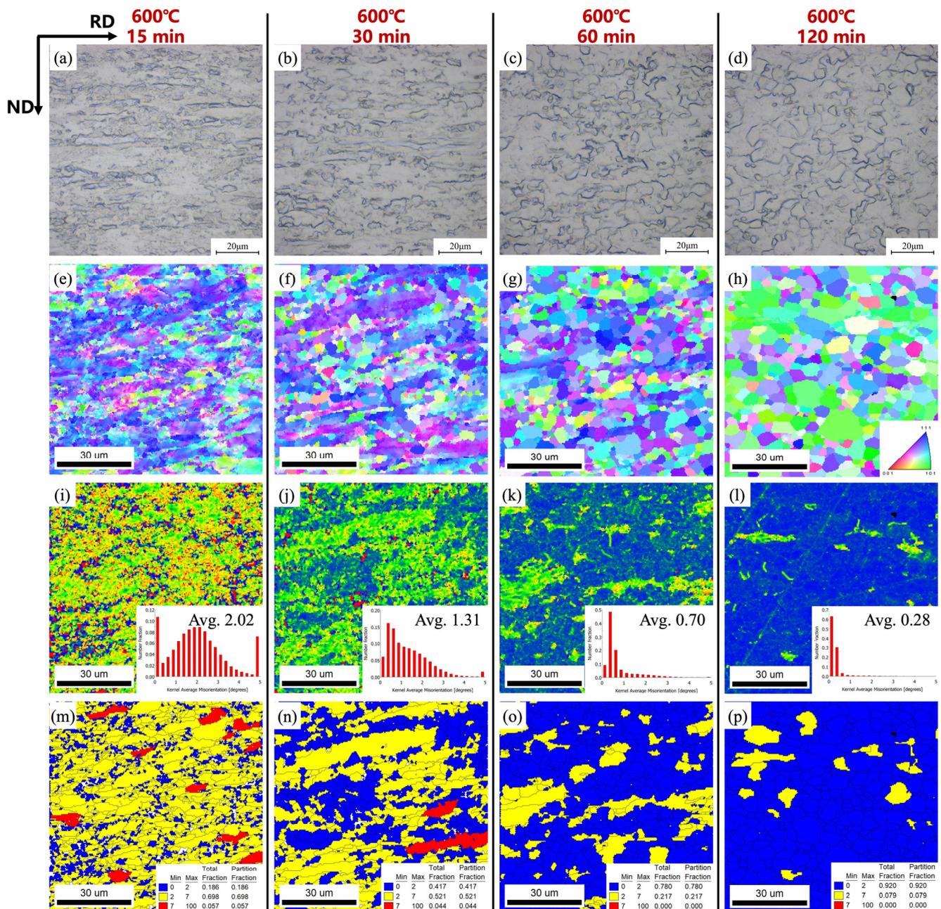
**Figure 5.** Microstructure and EBSD of  $\text{Ti}_{50}\text{Ni}_{47}\text{Fe}_3$  alloy annealed at 600 °C for different times. (a,e,i,m) Annealed for 15 min; (b,f,j,n) annealed for 30 min; (c,g,k,o) annealed for 60 min; (d,h,l,p)
