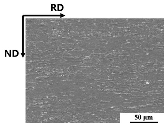
**Figure 1.** Microstructure of cold-rolled  $\text{Ti}_{50}\text{Ni}_{47}\text{Fe}_3$  alloy (RD for rolling direction, ND for normal direction).
