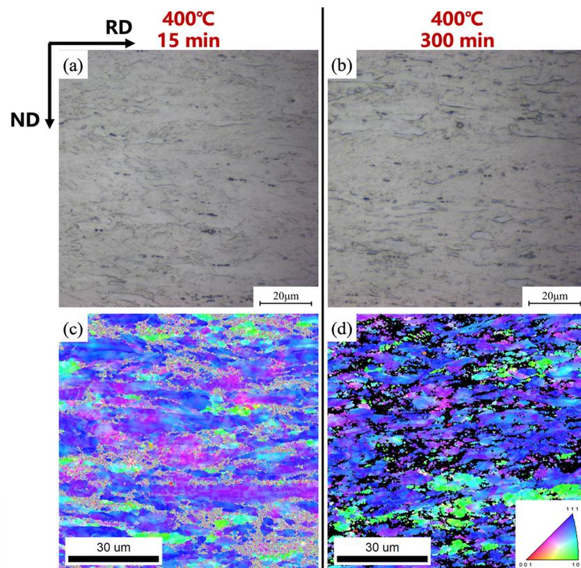
**Figure 3.** Microstructure and orientation analyses of TiNiFe alloy annealed at 400 °C for different times. (a,c) Annealed for 15 min; (b,d) annealed for 300 min. Among them, panels (a,b) are OM, and panels (c,d) are EBSD-IPF maps (the black area is an uncalibrated area that is difficult to calibrate due to the large amount of cold-working deformation, which is consistent with the uncalibrated areas in the other IPF maps).
