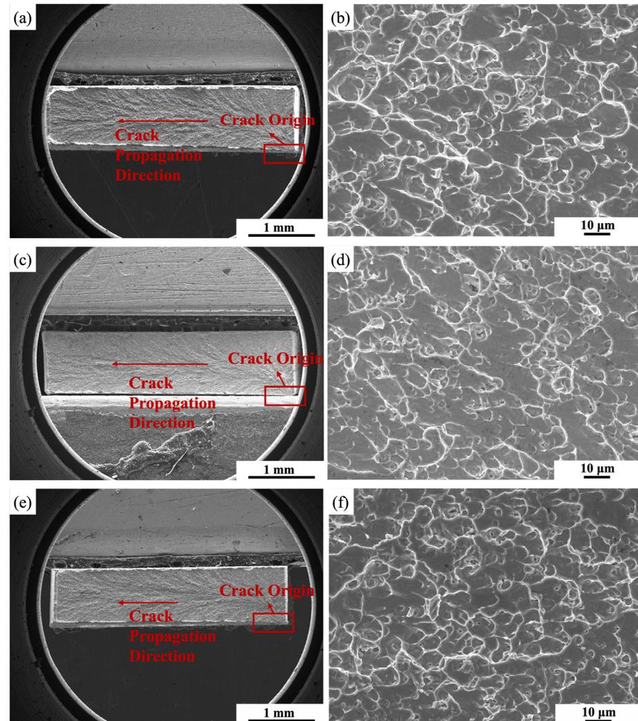
**Figure 10.** Fracture characteristics of  $\text{Ti}_{50}\text{Ni}_{47}\text{Fe}_3$  alloys. (a,b) Annealed at 400 °C for 300 min; (c,d) annealed at 500 °C for 300 min; (e,f) annealed at 600 °C for 300 min.
