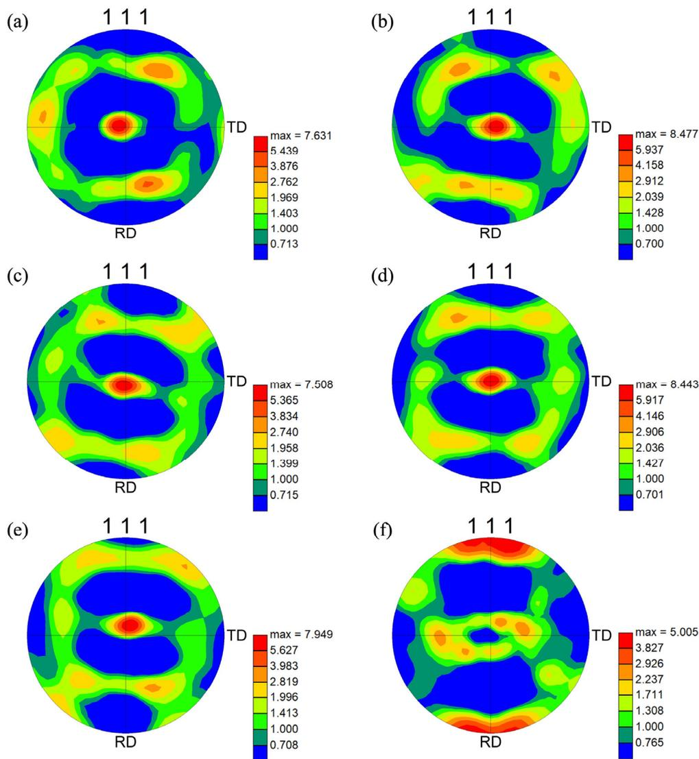
**Figure 7.** Pole figures (PFs) of  $\text{Ti}_{50}\text{Ni}_{47}\text{Fe}_3$  alloy with different annealing treatments. (a) Annealed at  $400\text{ }^\circ\text{C}$  for 15 min; (b) annealed at  $400\text{ }^\circ\text{C}$  for 300 min; (c) annealed at  $500\text{ }^\circ\text{C}$  for 15 min; (d) annealed at  $500\text{ }^\circ\text{C}$  for 300 min; (e) annealed at  $600\text{ }^\circ\text{C}$  for 15 min; (f) annealed at  $600\text{ }^\circ\text{C}$  for 120 min.
