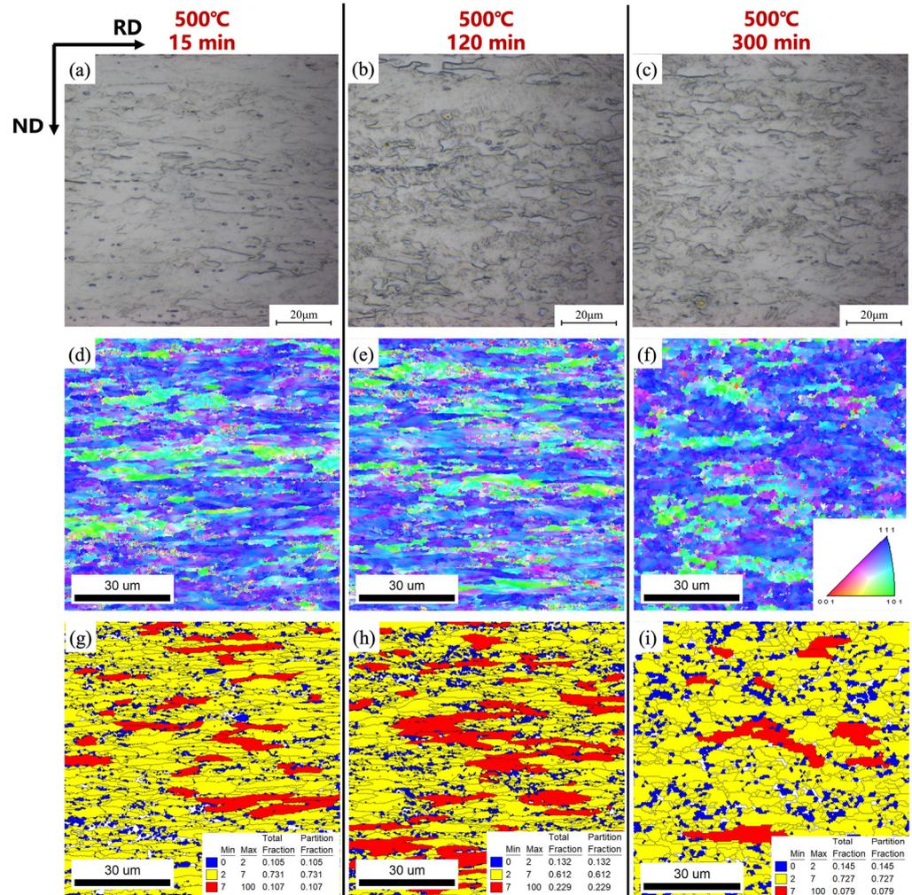
**Figure 4.** Microstructure and orientation analyses of  $\text{Ti}_{50}\text{Ni}_{47}\text{Fe}_3$  alloy annealed at 500 °C for different times. (a,d,g) Annealed for 15 min; (b,e,h) annealed for 120 min; (c,f,i) annealed for 300 min. Among them, panels (a–c) are OM images, panels (d–f) are EBSD-IPF maps, and panels (g–i) are EBSD-GOS maps.
