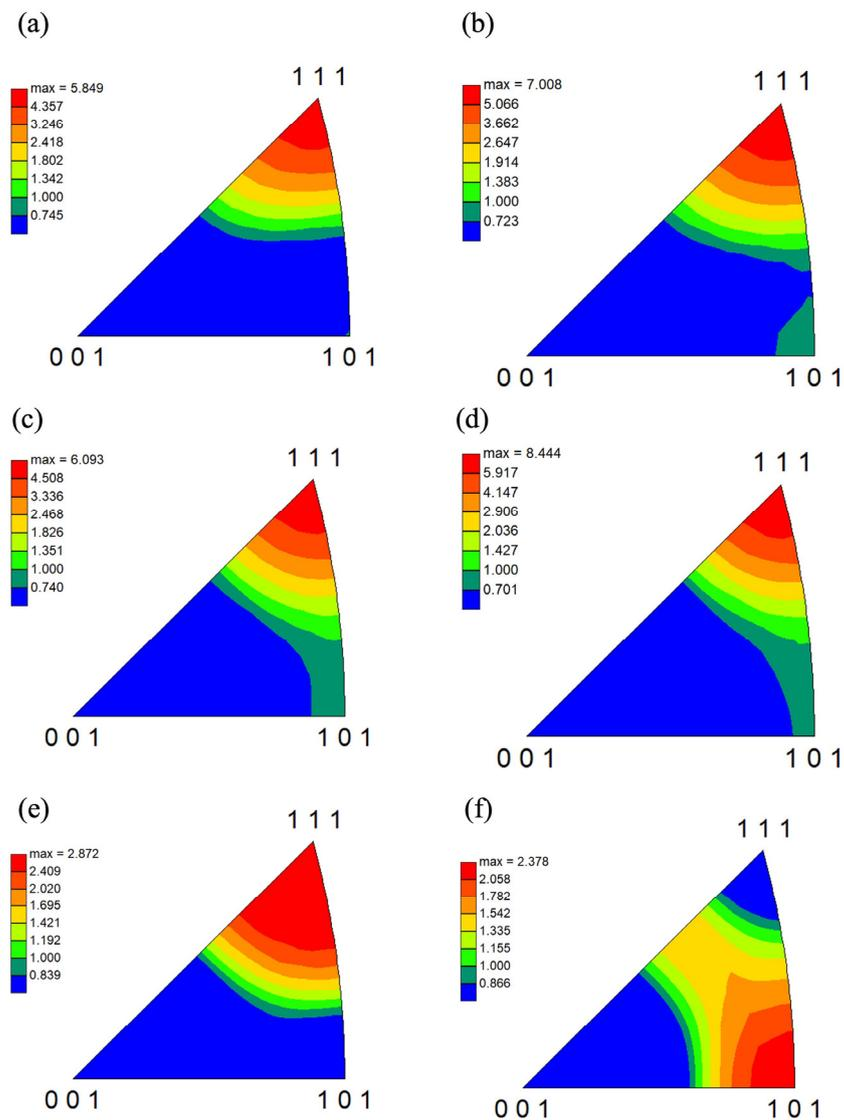
**Figure 6.** Inverse pole figures (IPFs) in the RD of  $Ti_{50}Ni_{47}Fe_3$  alloy with different annealing treatments. (a) Annealed at 400 °C for 15 min; (b) annealed at 400 °C for 300 min; (c) annealed at 500 °C for 15 min; (d) annealed at 500 °C for 300 min; (e) annealed at 600 °C for 15 min; (f) annealed at 600 °C for 120 min.
