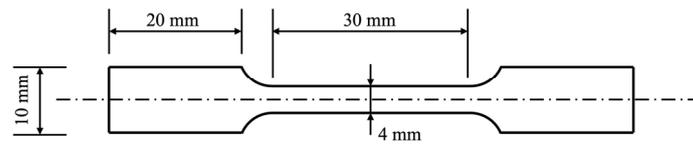
**Figure 2.** Schematic diagram of tensile test specimen.
