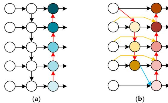
**Figure 6.** PANet and BiFPN structures. (a) PANet. (b) BiFPN. Notes: “○” denotes the network layer and “→” denotes the connection relationship between the network layers.
