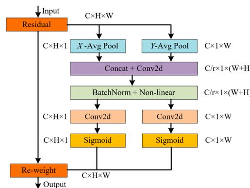
Figure 5. Structure of the coordinate attention module.
