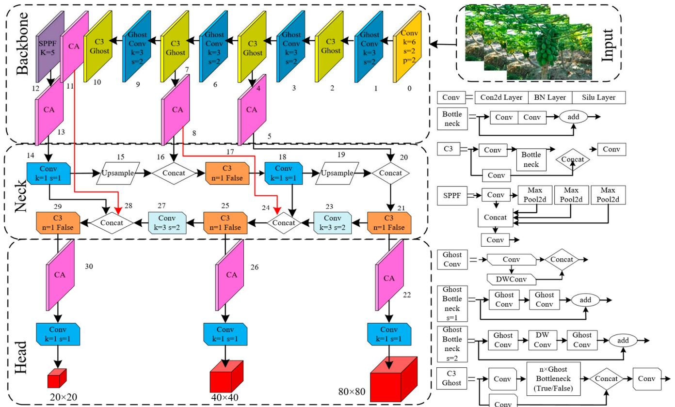
Figure 8. YOLOV5s-Papaya network structure.
