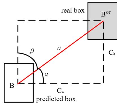
Figure 7. SIoU bounding box losses.
