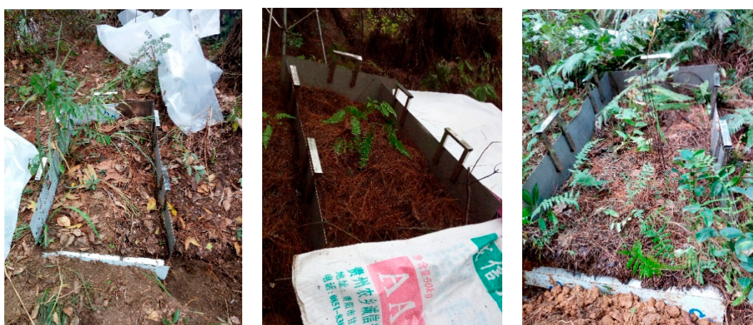
Figure 2. Micro-runoff plot setup in the forest.
