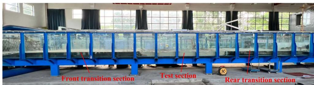
Figure 4. Experimental flume and sediment flume.
