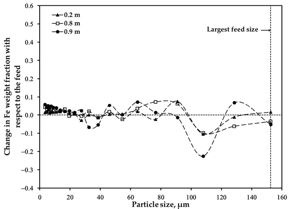
Figure 15. Changes in iron content in particles within the unsieved concentrate oxidized under 70 pct. O<sub>2</sub> in the process gas.
