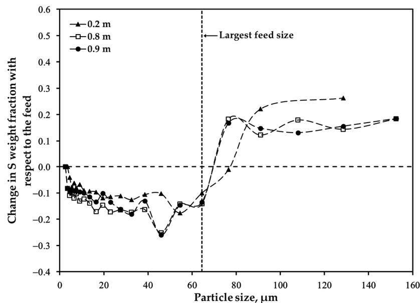
**Figure 10.** Changes in sulfur content in particles within the size fraction of  $<45 \mu\text{m}$  oxidized under 70 pct.  $\text{O}_2$  in the process gas.
