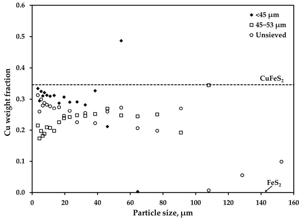
Figure 5. Copper content in the sieved fractions and unsieved La Caridad copper concentrate particles.
