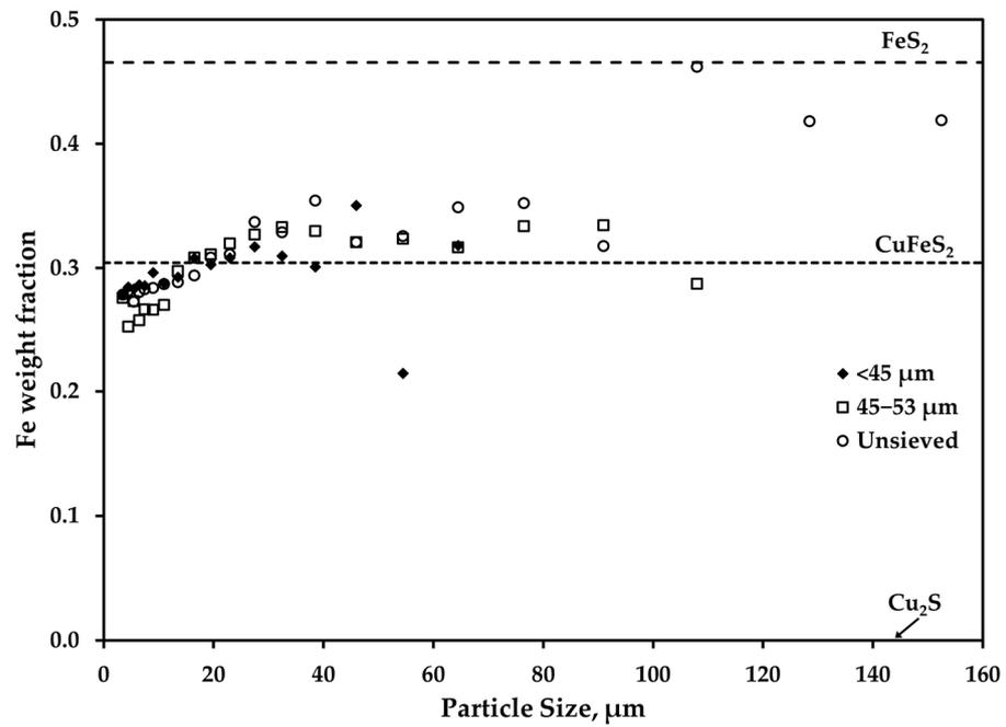
Figure 6. Iron content in the sieved fractions and unsieved La Caridad copper concentrate particles.
