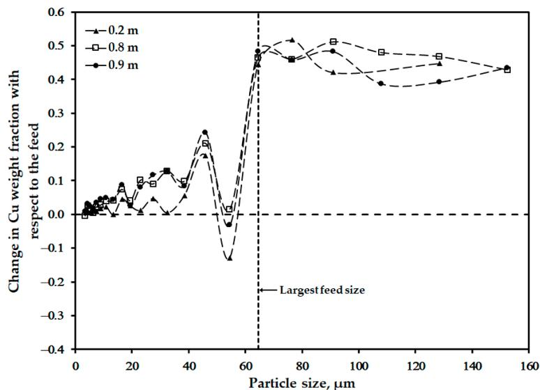
**Figure 8.** Changes in copper content in particles within the size fraction of <45 μm oxidized under 70 pct. O<sub>2</sub> in the process gas.
