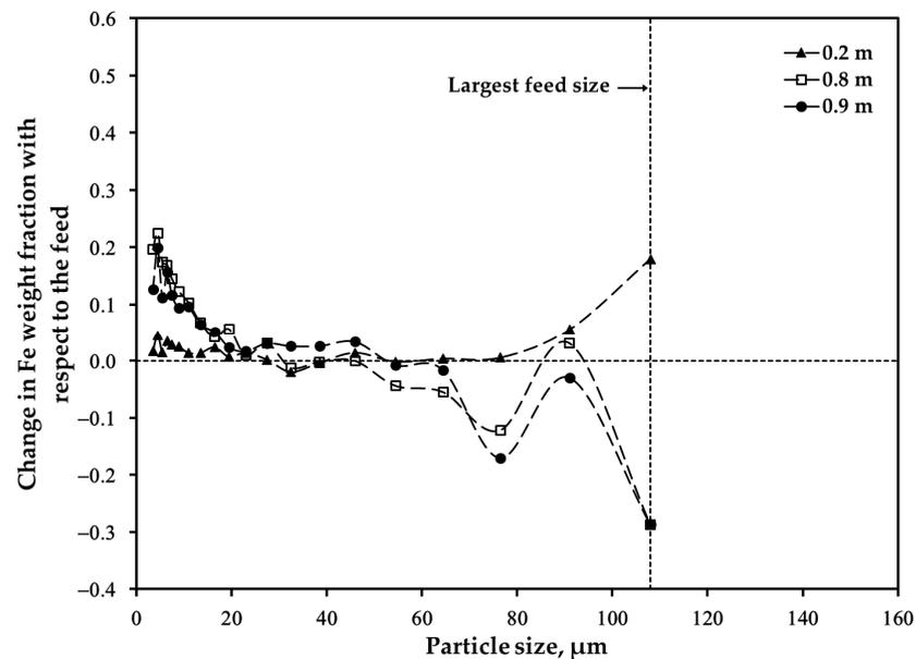
**Figure 12.** Changes in iron content in particles within the size fraction of 45–53  $\mu\text{m}$  oxidized under 70 pct.  $\text{O}_2$  in the process gas.
