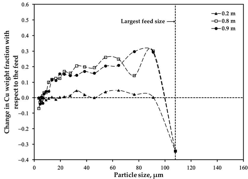
**Figure 11.** Changes in copper content in particles within the size fraction of 45–53  $\mu\text{m}$  oxidized under 70 pct.  $\text{O}_2$  in the process gas.
