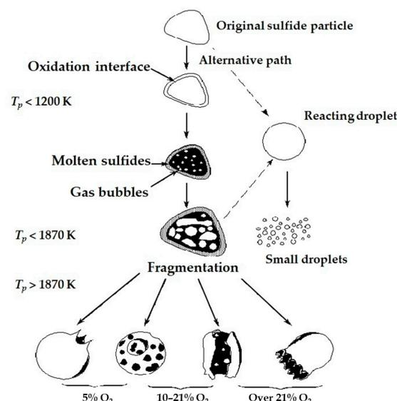
**Figure 1.** Reaction path of sulfide particles during flash smelting assuming low density of the particle–gas suspension. Adapted from references [9,15].
