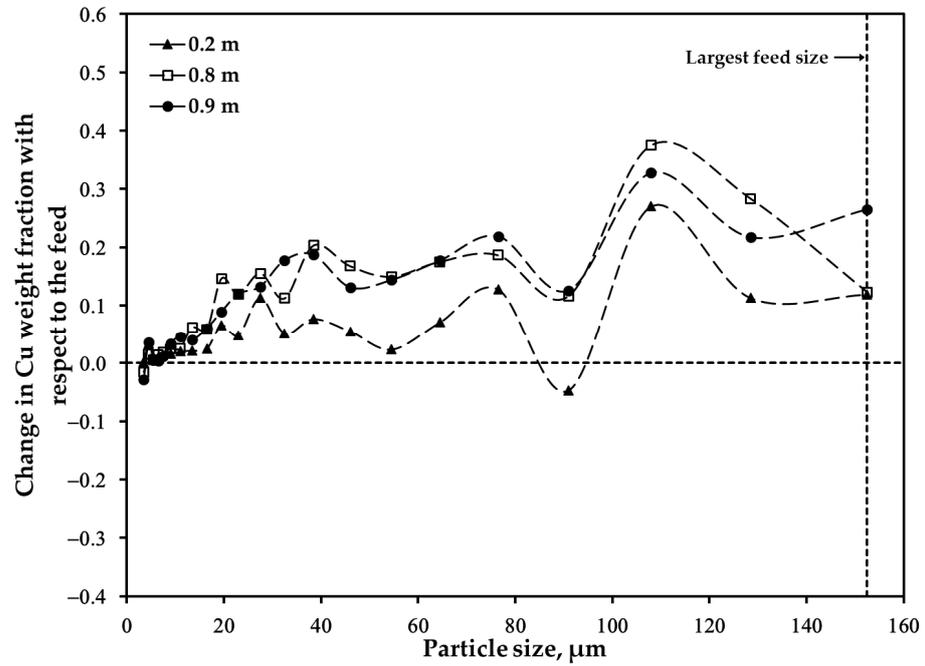
Figure 14. Changes in copper content in particles within the unsieved concentrate oxidized under 70 pct. O<sub>2</sub> in the process gas.
