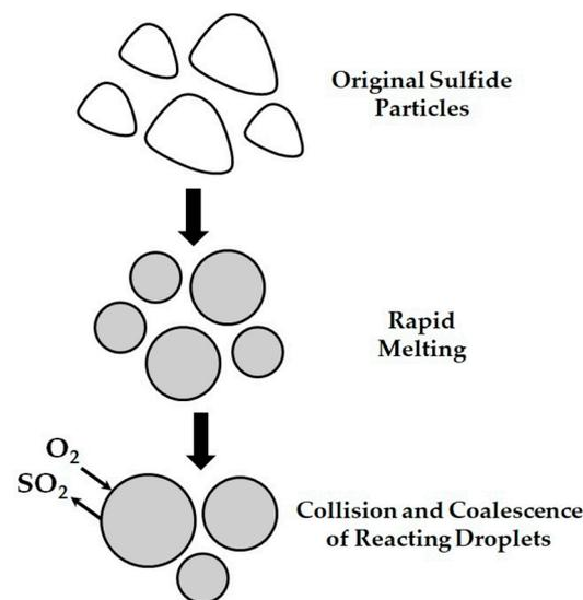
**Figure 2.** Reaction path of sulfide particles during flash smelting assuming high density of the particle–gas suspension. Adapted from references [14,16].
