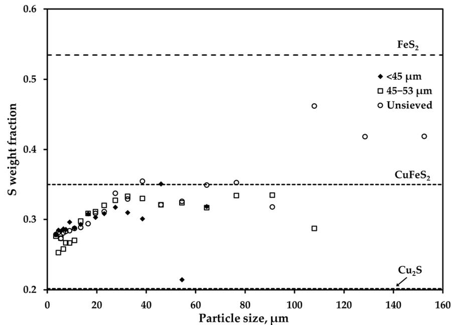
**Figure 7.** Sulfur content in the sieved fractions and unsieved La Caridad copper concentrate particles.
