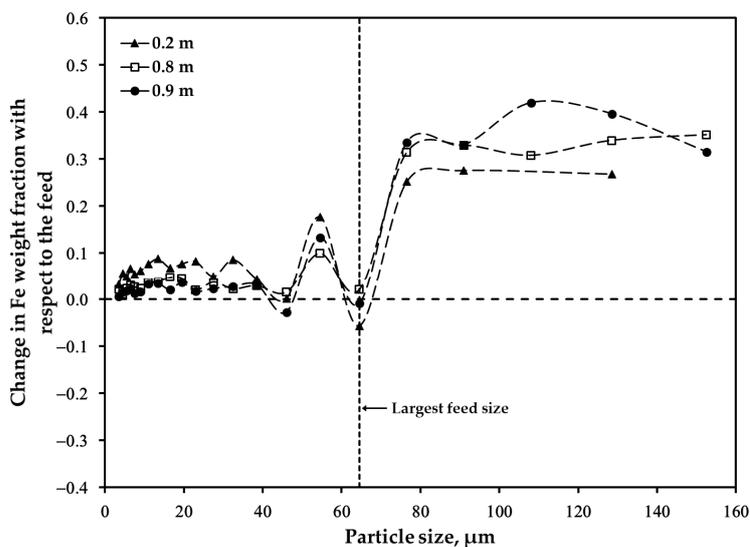
**Figure 9.** Changes in iron content in particles within the size fraction of <45 μm oxidized under 70 pct. O<sub>2</sub> in the process gas.
