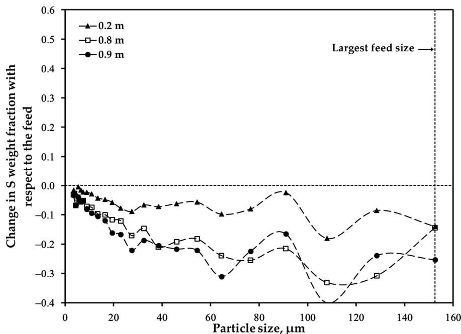
**Figure 16.** Changes in sulfur content in particles within the unsieved concentrate oxidized under 70 pct.  $O_2$  in the process gas.
