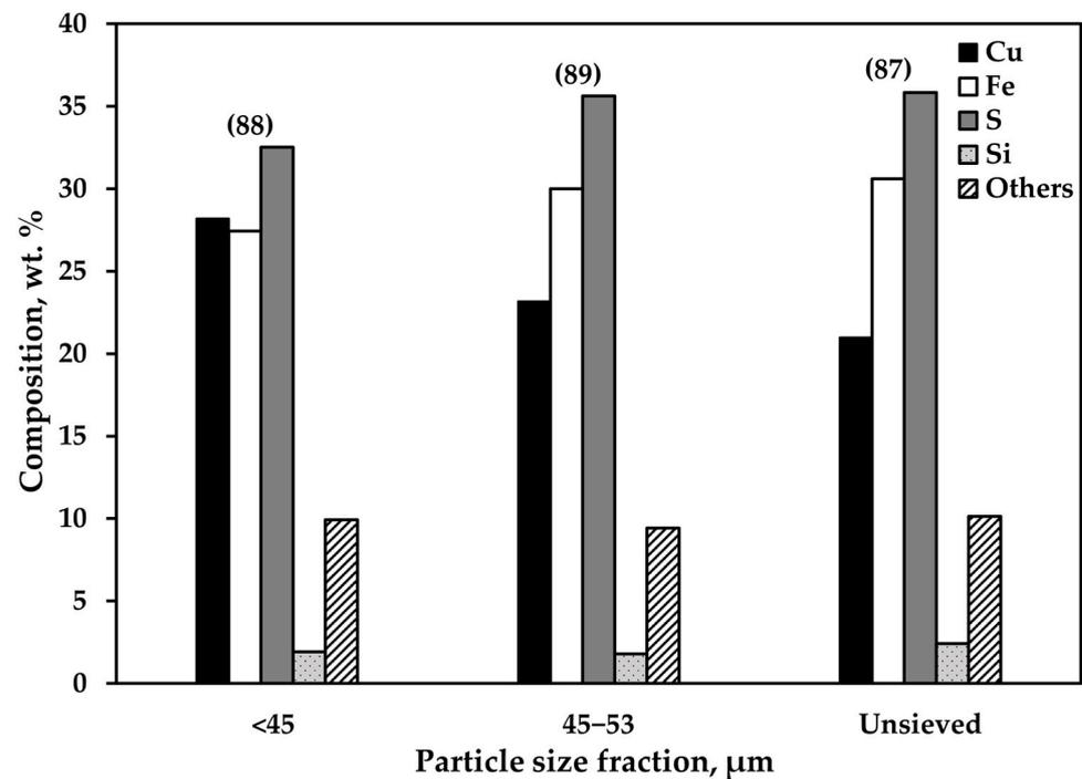
**Figure 3.** Overall chemical compositions of size fractions of <45 μm and 45–53 μm and the unsieved concentrate. The values in parentheses represent the summation of copper, iron, and sulfur contents.
