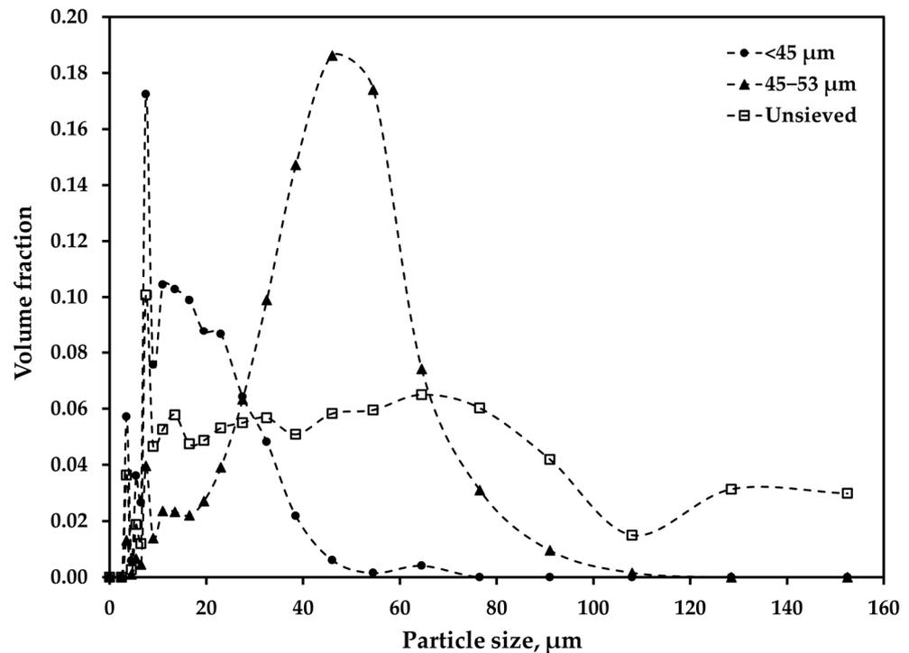
**Figure 4.** Particle size distributions of size fractions of <45  $\mu\text{m}$  and 45–53  $\mu\text{m}$  and unsieved concentrate determined by the QEMSCAN<sup>®</sup> unit.
