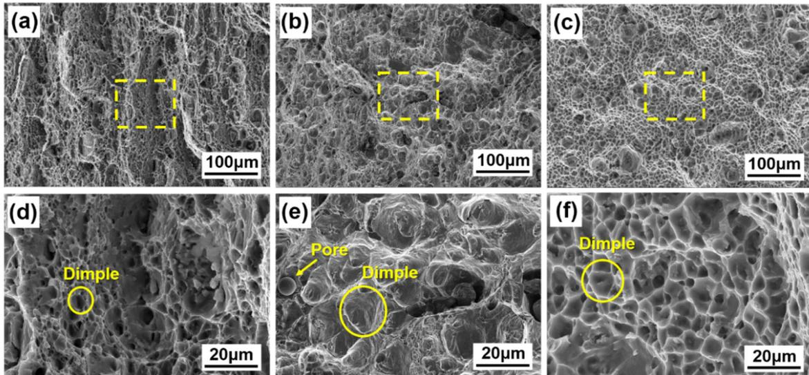
**Figure 14.** The fractured surface of different Al alloy joints: (a) and (d) for 5083; (b) and (e) for 6005A; (c) and (f) for 7N01.
