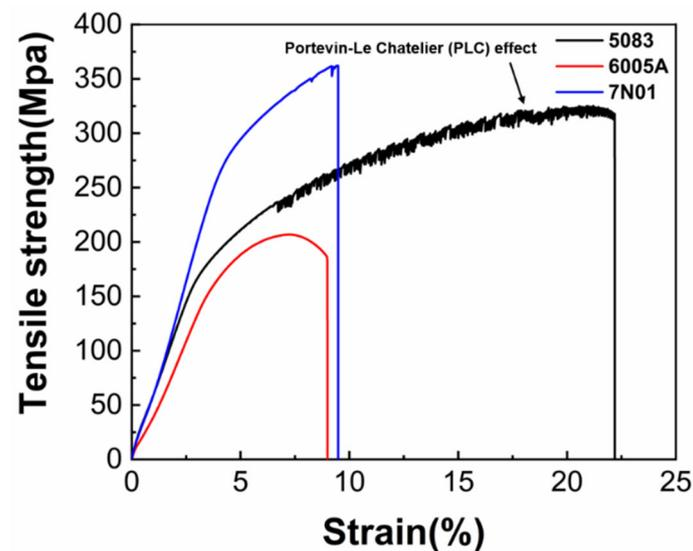
**Figure 12.** The displacement-strength curves of 5083, 6005A and 7N01 Al alloys welded joints.
