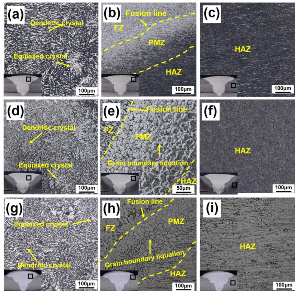
**Figure 4.** The microstructure of different aluminum alloy welded joints: 5083: (a) fusion zone (FZ), (b) partially melted zone (PMZ), (c) heat-affected zone (HAZ); 6005A: (d) FZ, (e) PMZ, (f) HAZ; 7N01: (g) FZ, (h) PMZ, (i) HAZ.
