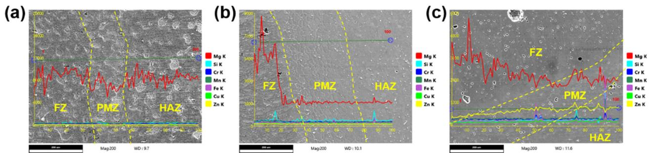
**Figure 5.** Energy-dispersive X-ray spectroscopy (EDS) scanning results of different aluminum alloy welded joints: (a) 5083; (b) 6005A; (c) 7N01.
