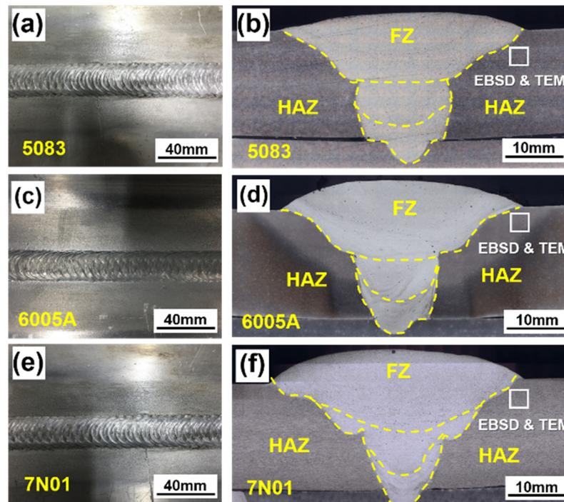
**Figure 3.** The weld appearance and cross section of welding joints: (a,b) for 5083; (c,d) for 6005A; (e,f) for 7N01.
