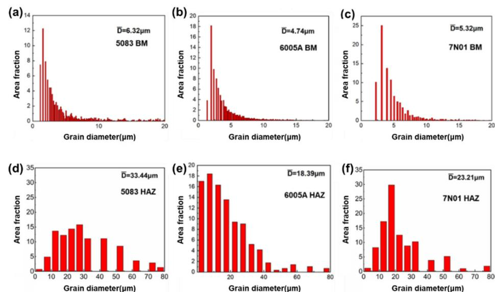
**Figure 8.** The grain size of different aluminum alloy welded joints: 5083: (a) BM; (b) HAZ; 6005A: (c) BM; (d) HAZ; 7N01: (e) BM; (f) HAZ.
