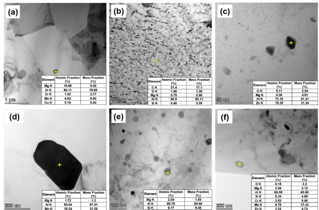
**Figure 9.** EDS results of different aluminum alloy welded joints: 5083: (a) BM; (d) HAZ; 6005A: (b) BM; (e) HAZ; 7N01: (c) BM, (f) HAZ.
