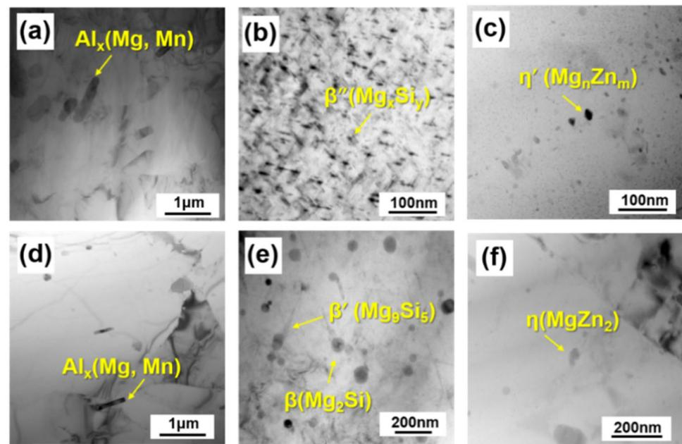
**Figure 10.** Bright-field transmission electron microscopy (TEM) micrograph of different aluminum alloy welded joints: 5083: (a) BM; (d) HAZ; 6005A: (b) BM; (e) HAZ; 7N01: (c) BM, (f) HAZ.
