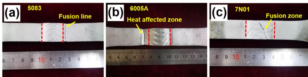
**Figure 13.** Fracture position of different aluminum alloy welded joints: (a) 5083; (b) 6005A; (c) 7N01.
