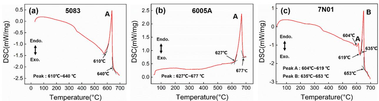
**Figure 6.** The differential scanning calorimetry (DSC) curves of different aluminum alloy joints: (a) 5083; (b) 6005A; (c) 7N01.
