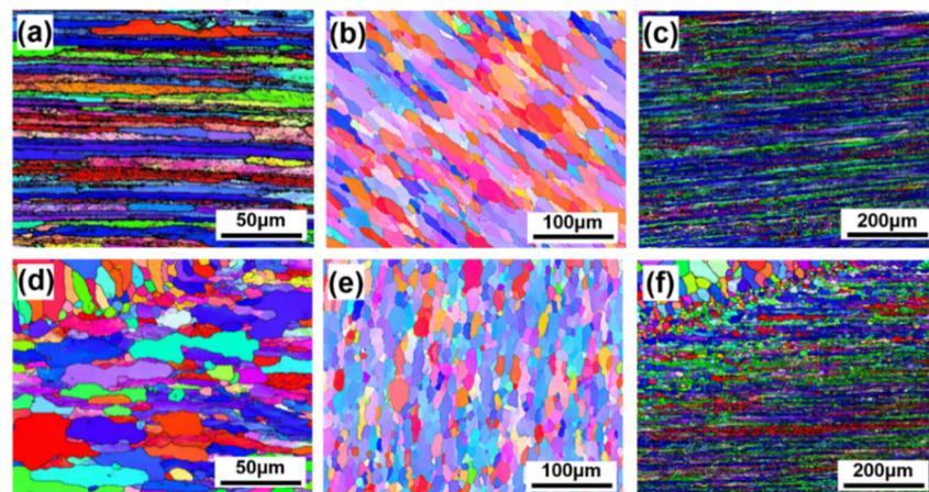
**Figure 7.** Electron backscatter diffraction detector (EBSD) images of aluminum alloy welding joints: 5083: (a) base metal (BM); (d) HAZ; 6005A: (b) BM; (e) HAZ; 7N01: (c) BM; (f) HAZ.
