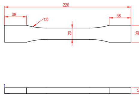
**Figure 2.** Geometry of the tensile specimens (mm).
