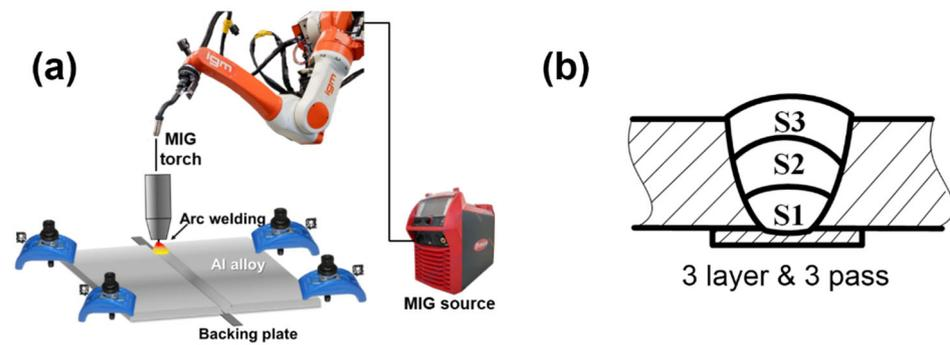
**Figure 1.** The schematic of gas metal arc welding (GMAW) of aluminum alloy. (a) welding diagram; (b) three-layer and three-pass welding layer arrangement.
