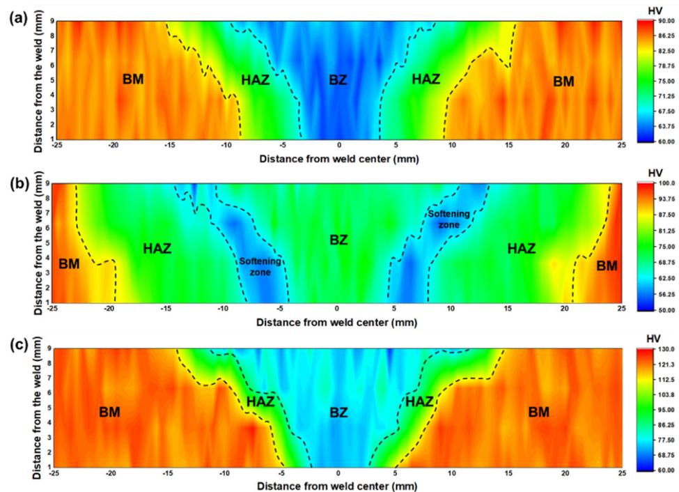
**Figure 11.** Microhardness profile of different aluminum alloy welded joints: (a) 5083; (b) 6005A; (c) 7N01.
