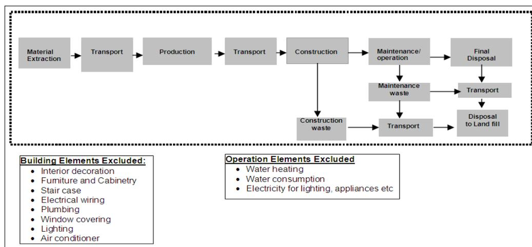
**Figure 1.** LCA system boundary.
