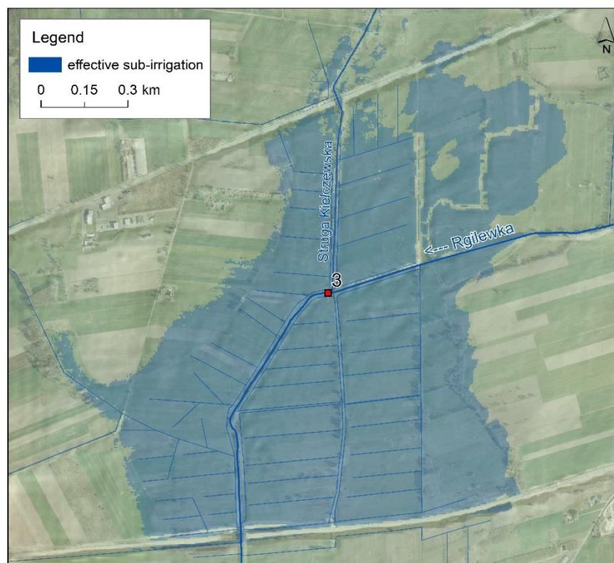
**Figure 6.** The range of the impact of water damming on weir No. 3 at km 11 + 371 of the Rgilewka River on the adjacent land (range of effective irrigation).
