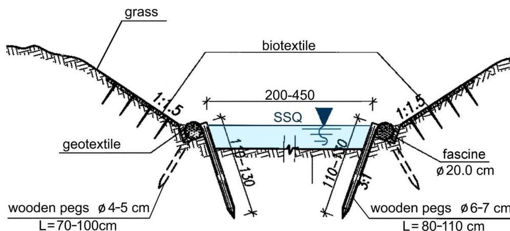
**Figure 5.** Cross-section through the river channel, presenting the fortification in the vicinity of rebuilt weirs on the Rgilewka River (source: [20]—changed).
