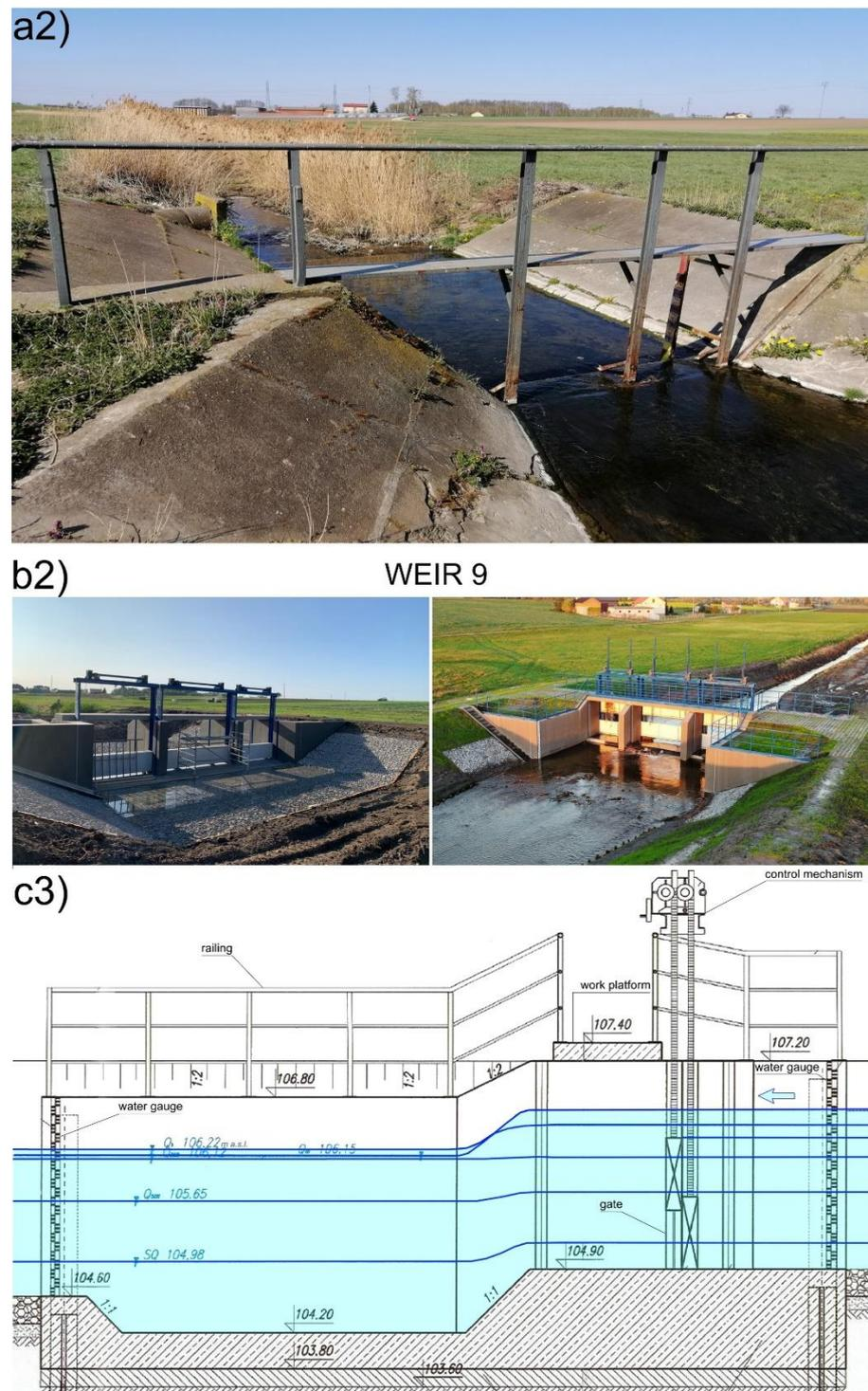
**Figure 3.** Example reconstruction of weirs (weir No. 7 and weir No. 9) on the Rgilewka River: (a1,a2) original state, (b1,b2) present state, and (c1,c3) longitudinal cross-section (source: [20]—changed).
