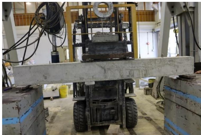
Figure 5. Experimental setup of RC beam specimen.
