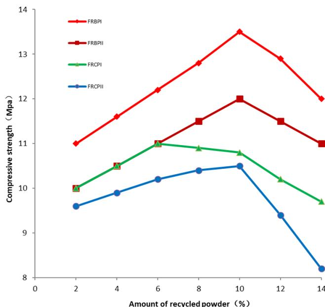
**Figure 5.** Compressive strength of adobe material mixed with recycled powder and cured at normal temperature for 28 days.
