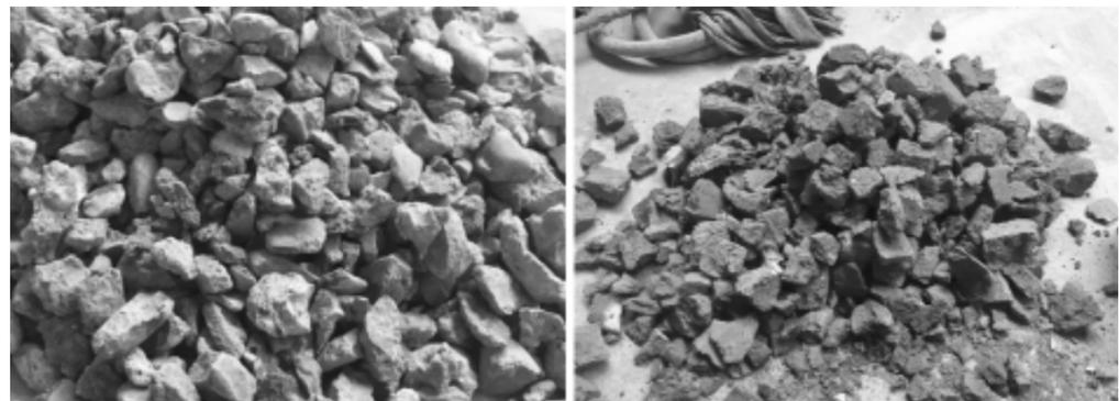
**Figure 2.** Waste concrete coarse aggregate (left) and waste brick coarse aggregate (right).
