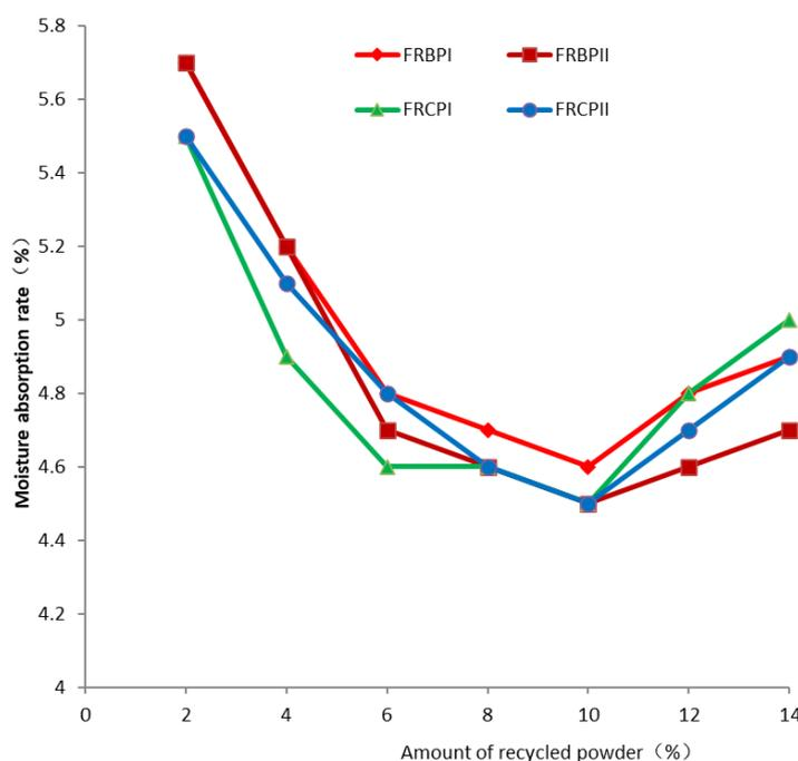
**Figure 7.** Experiment results of moisture absorption and desorption performance of adobe materials.
