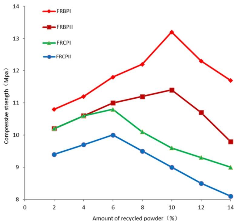
**Figure 6.** Compressive strength of adobe material mixed with recycled powder after 28 days of hot curing.
