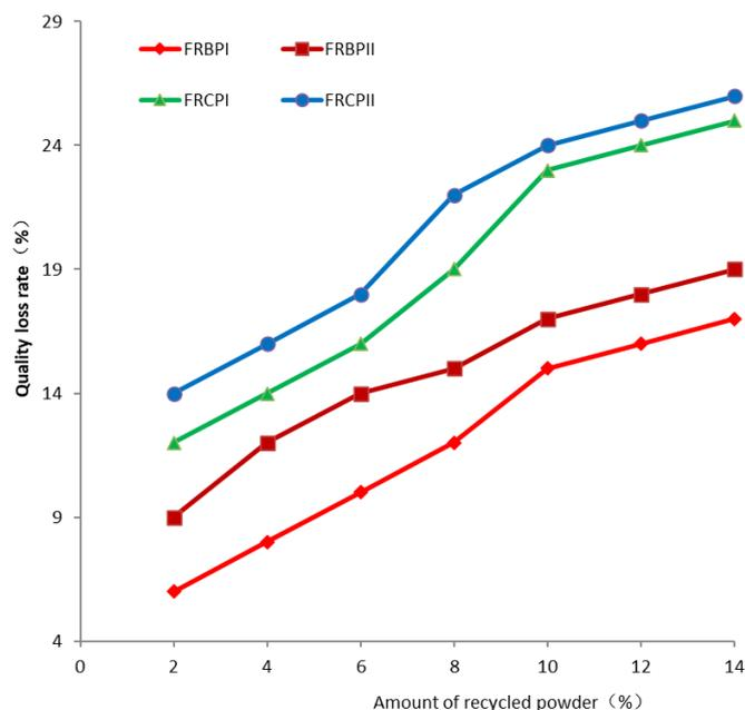
**Figure 8.** Experiment results of dry–wet cycle performance of adobe materials.
