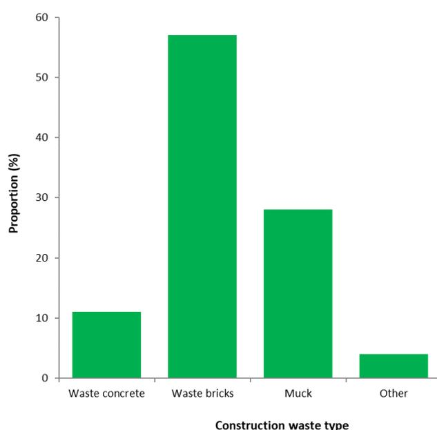
**Figure 1.** Proportion of various construction wastes.
