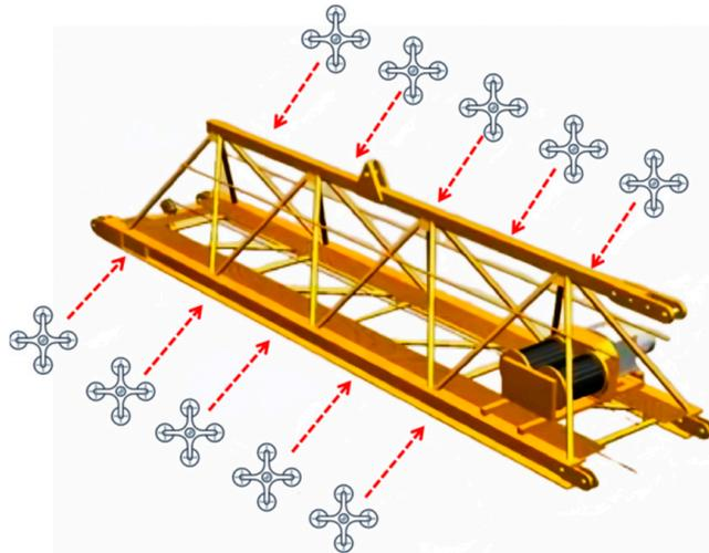
**Figure 2.** Flight path planning for tower crane boom.
