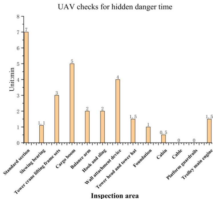
**Figure 13.** Time consumption of UAV intelligent inspection.
