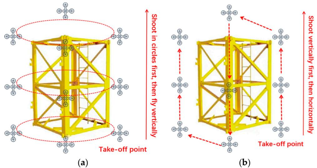
**Figure 1.** Standard section flight path planning for tower cranes. (a) Surrounding flight route. (b) Elevated flight route.
