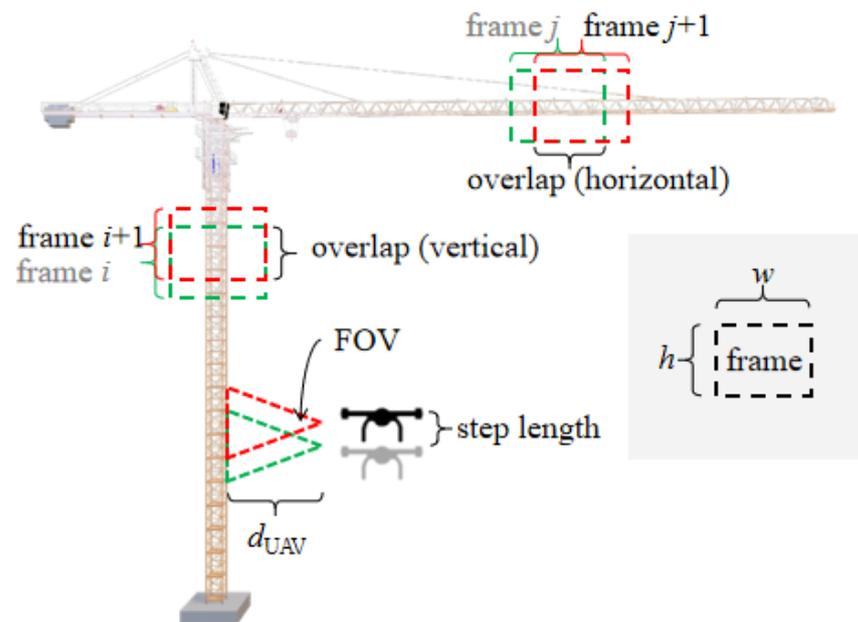
**Figure 3.** Illustration of scales used to determine the step length to take images.
