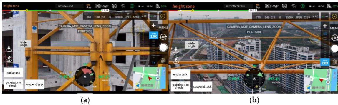
Figure 9. Operating interface of the UAV intelligent inspection application. (a) Automated shooting of the standard sections by UAV. (b) Automated shooting of the tower crane boom by UAV.
