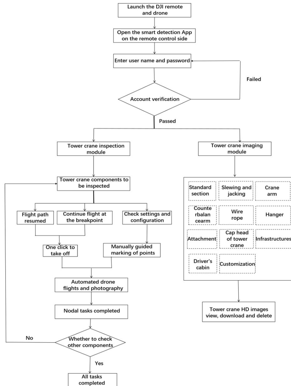
**Figure 5.** The operation procedure of the UAV intelligent inspection system.
