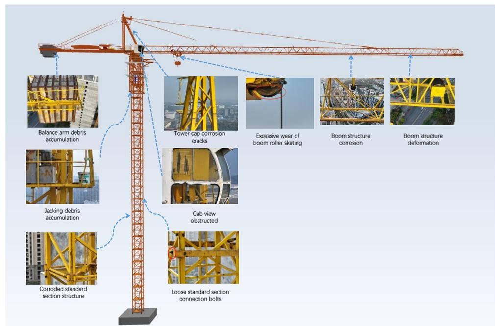
Figure 10. Photos of typical tower crane flaws taken by UAV.
