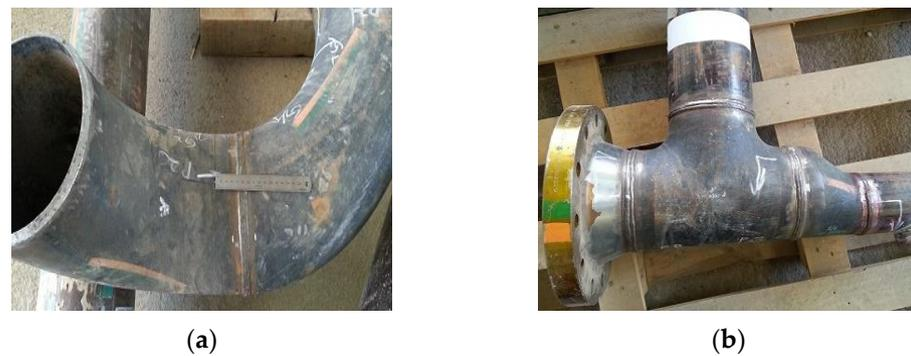
**Figure 1.** Piping and fitting with various curvature structures: (a) elbow; (b) flange and reducer.
