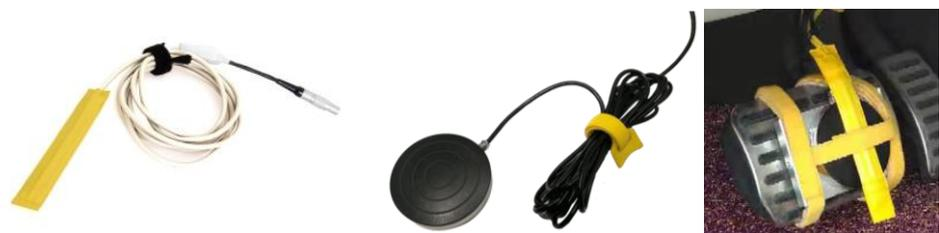
**Figure 3.** Brake trigger, pedal force sensor and installation style.
