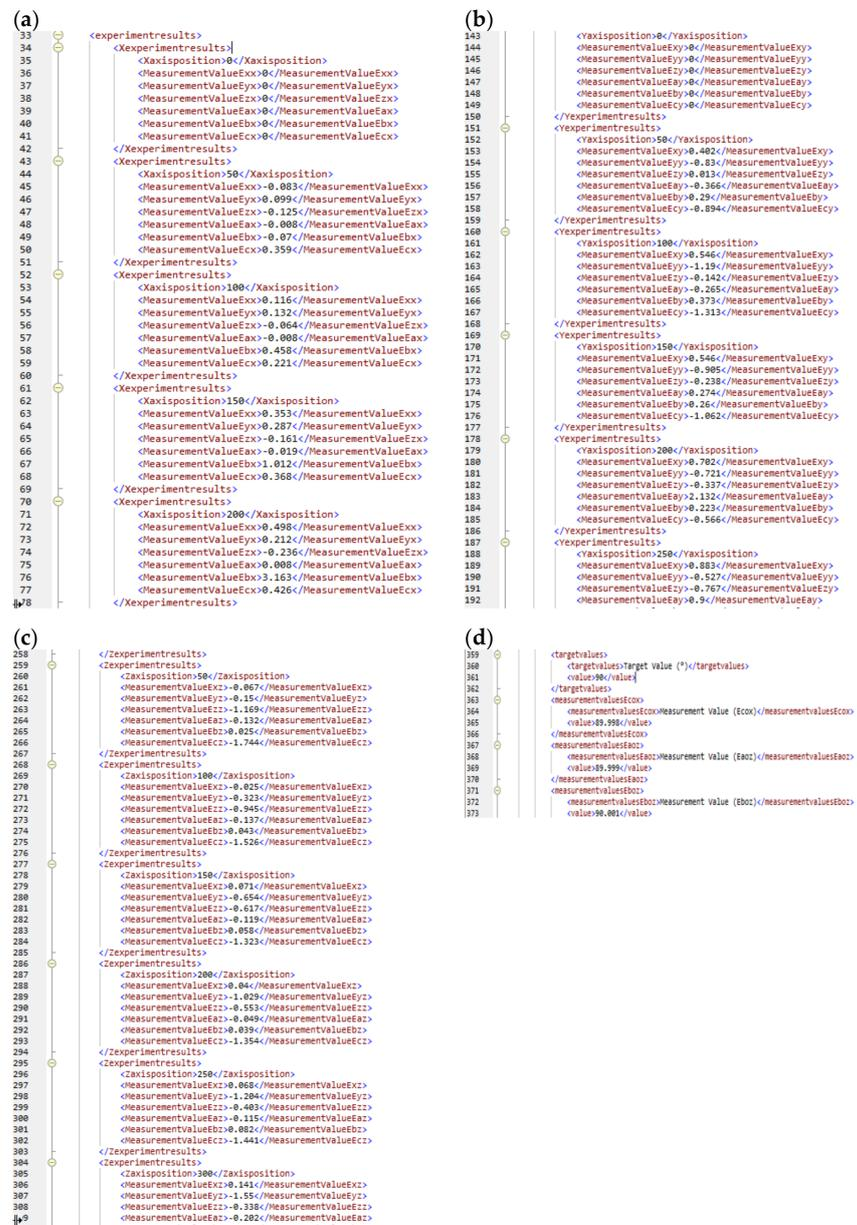
Figure 8. Measurement results of (a) X-axis, (b) Y-axis, (c) Z-axis, and (d) Squareness error of CMM in XML type.
