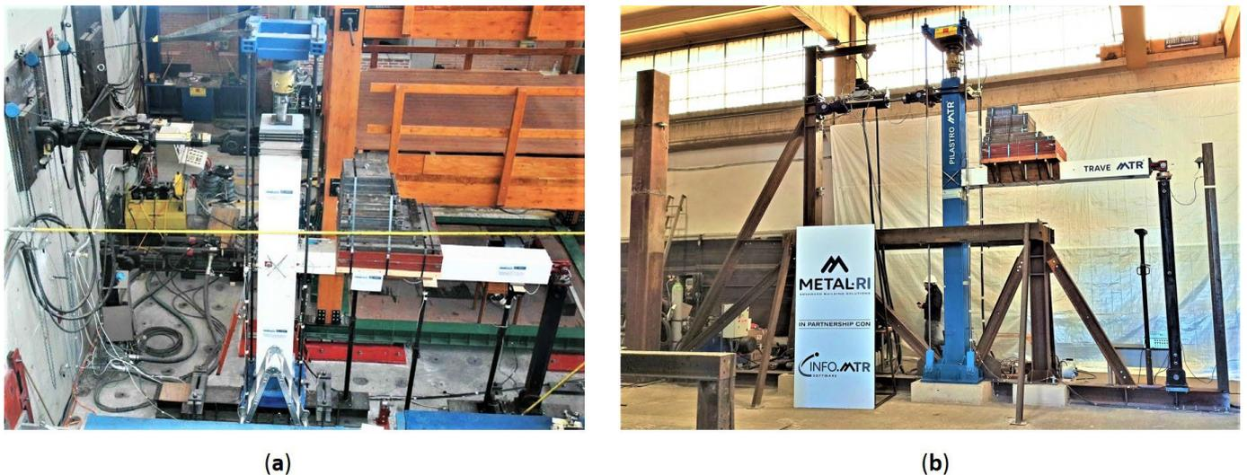
**Figure 3.** Test specimens: (a) hinged column model and (b) fixed column model.
