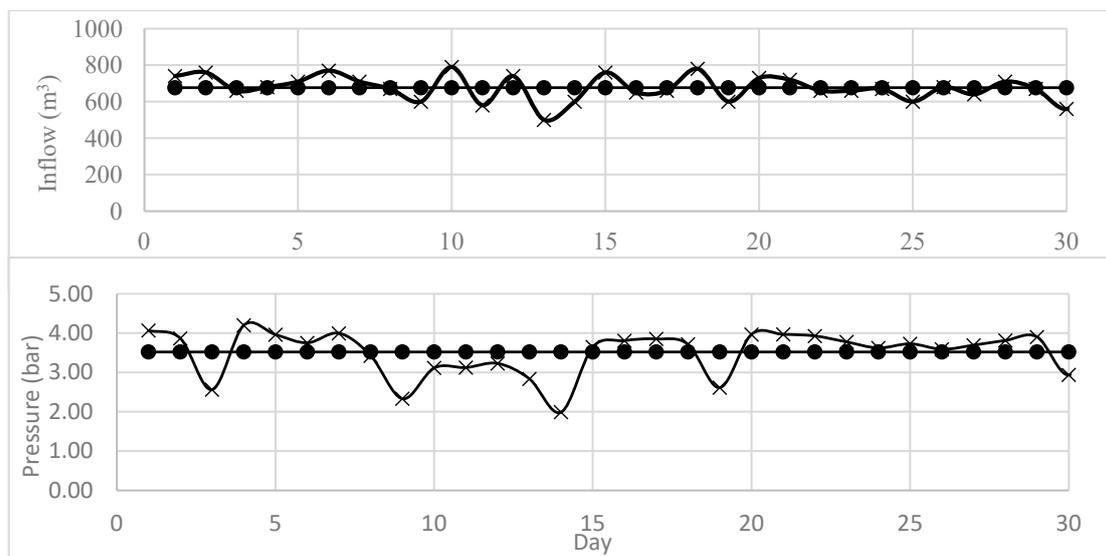
**Figure 2.** Flows (m<sup>3</sup>) and pressures (bar) per day in DMA 1, the straight line represents the average.
