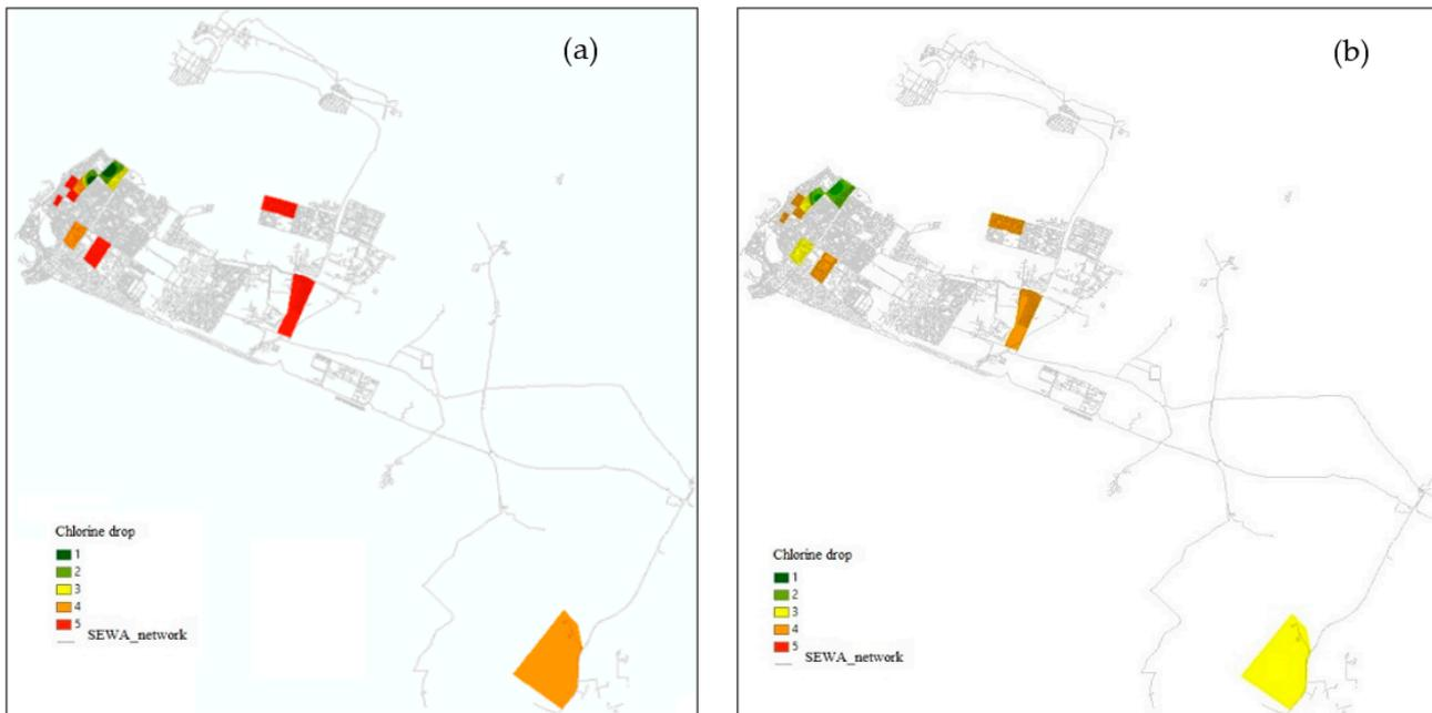
Figure 8. Chlorine drops maps. (a) Highest chlorine drop; (b) lowest chlorine drop.
