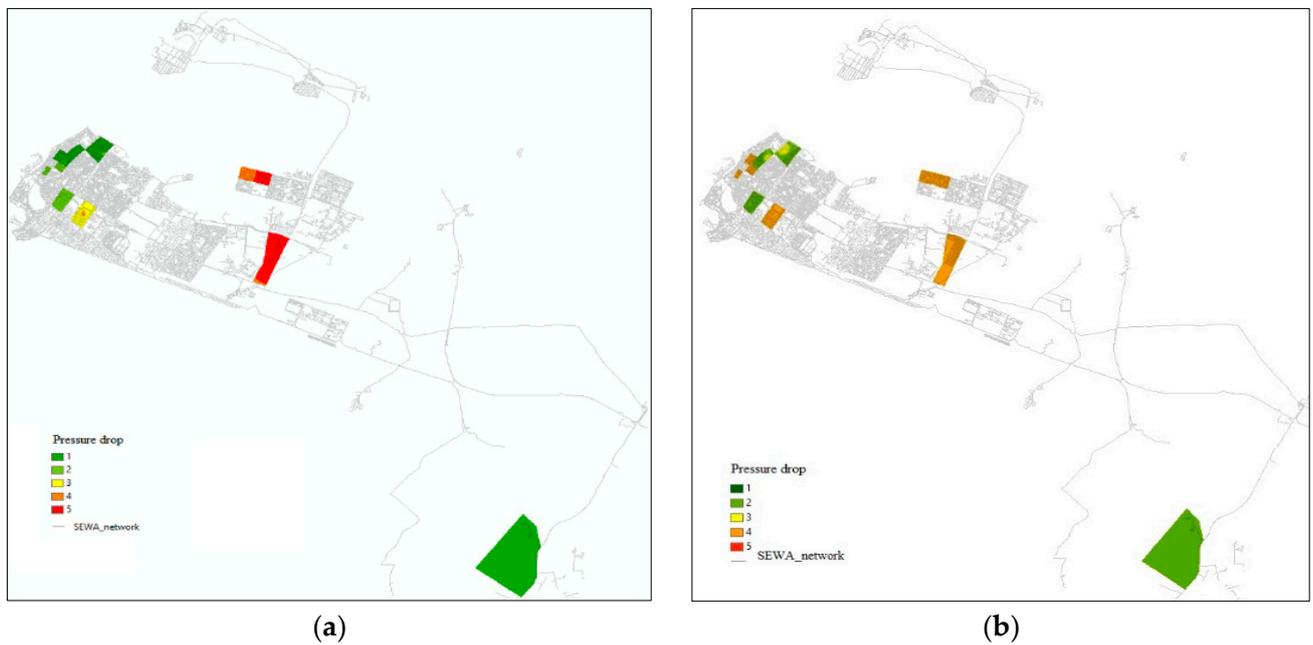
Figure 7. Pressure drops maps. (a) Highest pressure drop; (b) lowest pressure drop.
