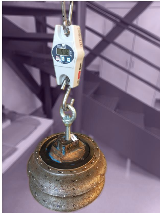
**Figure 6.** Weighing the worn disc cutter using a digital hanging scale.
