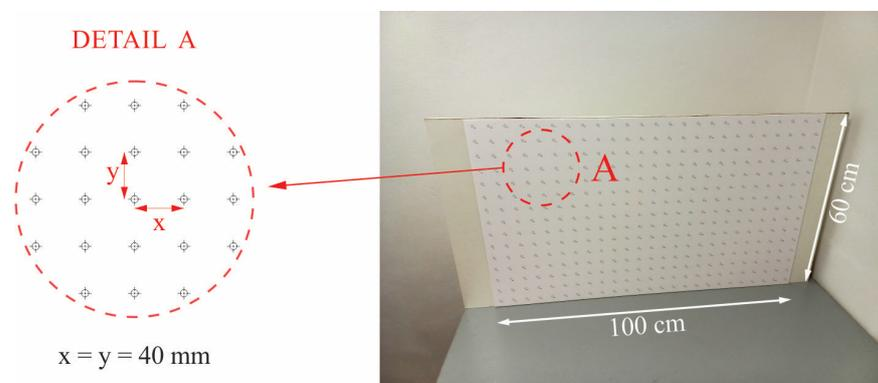
**Figure 7.** A background plate with targets used for close-range photogrammetry of the worn double disc cutter.
