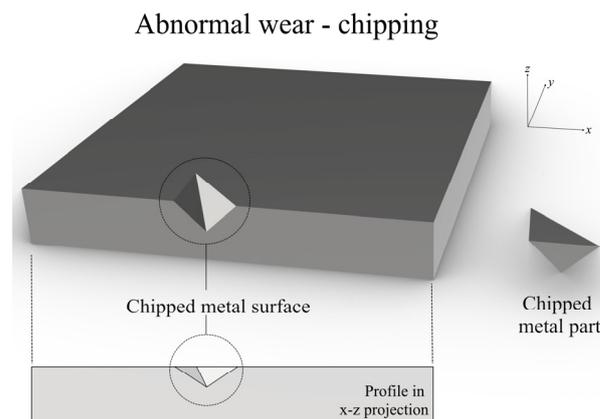
**Figure 2.** Schematic representation of material chipping, one of the abnormal types of wear in TBM disc cutters.
