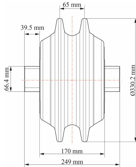
**Figure 4.** Technical drawing of the new double disc cutter.
