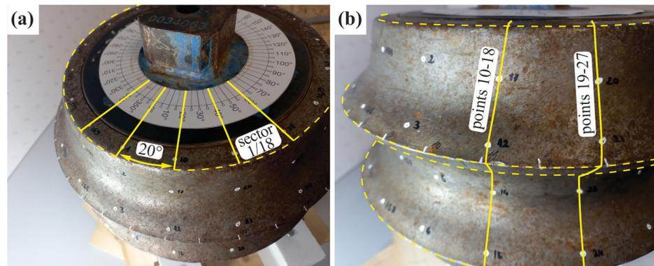
**Figure 8.** Marker points on the disc cutter's surface. (a) Sectors on the upper cutter ring; (b) detail of a sector with marker points on the boundary lines.
