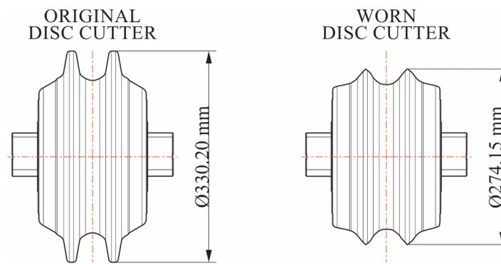
**Figure 14.** Original cross-section ( $\text{Ø}$  330.2 mm) and worn cross-section ( $\text{Ø}$  274.2 mm) of the double disc cutter.
