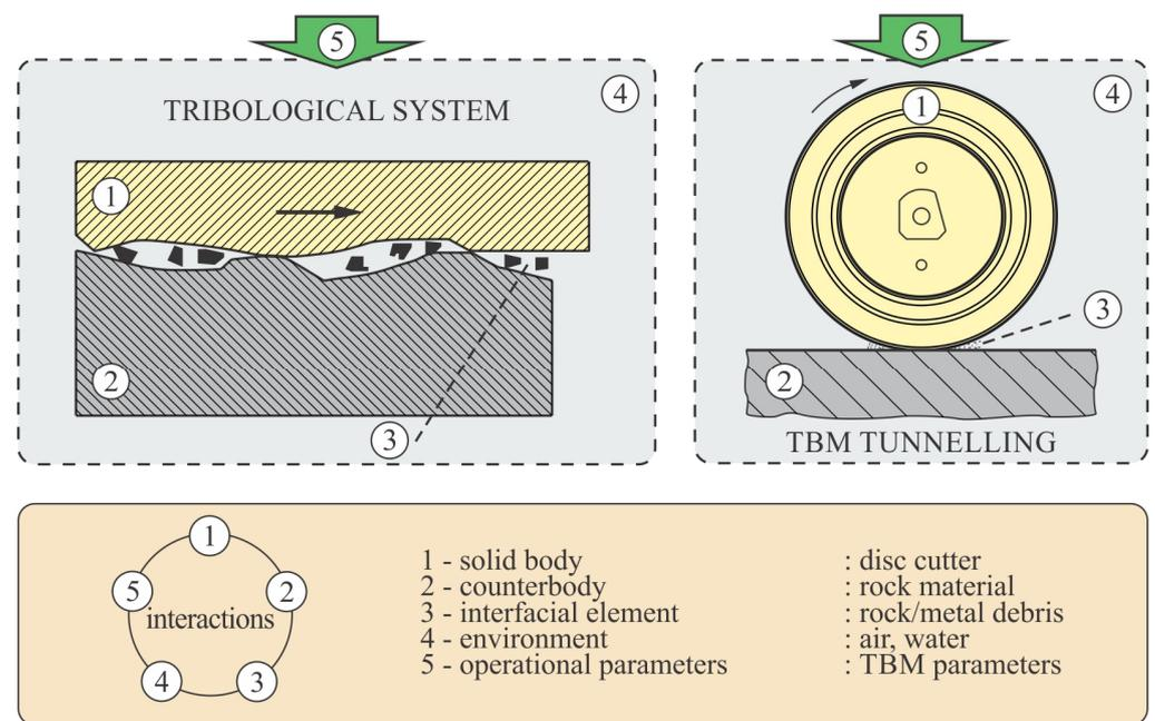
**Figure 3.** Tribological system with key components in the case of TBM tunneling.
