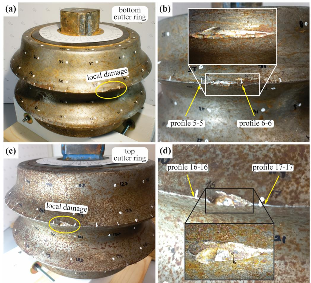
**Figure 10.** Local damages on the lower (bottom) and upper (top) cutter ring surface. (a) Area of localized damage on the bottom cutter ring of the double disc cutter, (b) enlarged view of the damage between profiles 5–5 and 6–6, (c) area of localized damage on the upper (top) cutter ring of the double disc cutter, and (d) enlarged view of the damage between profiles 16–16 and 17–17.
