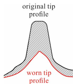
**Figure 15.** Detailed view of the original profile (top—black) and the worn profile (bottom—red) of cutter ring tip reconstructed from the point cloud. The worn surface of the profile is hatched.
