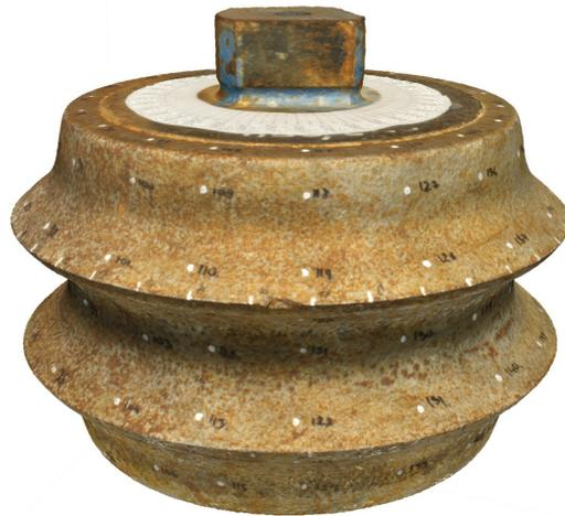
**Figure 13.** A 3D model of a worn disc cutter, created in Agisoft Metashape 1.6.3 software.
