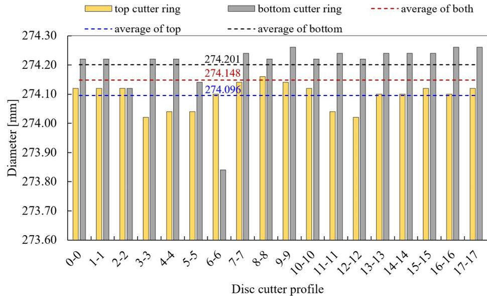
**Figure 11.** Diagram showing the diameters of the upper (yellow) and lower (grey) cutter rings of the double disc cutter measured using a caliper.
