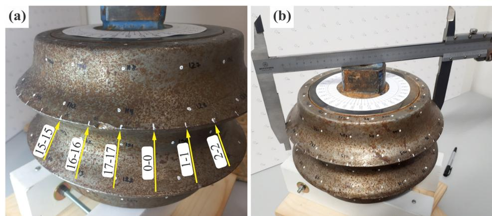
**Figure 5.** Measuring the diameter with a manual caliper. (a) Labeled profiles on the upper cutter ring (top); (b) the method of manually measuring the diameter with a caliper. Note that the white dots on the surface of the disc cutter were used for close-range photogrammetry.
