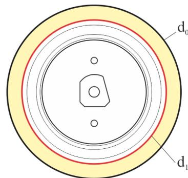
**Figure 12.** Original ( $d_0$ ) and average worn ( $d_1$ ) diameters of the double disc cutter. The worn surface is colored yellow.
