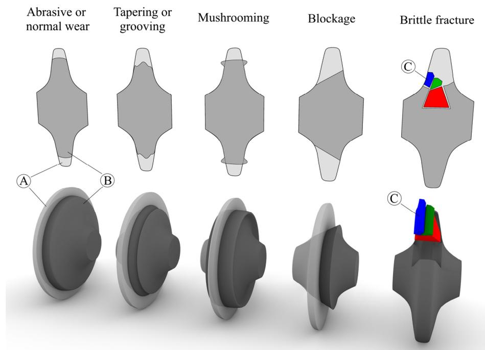
**Figure 1.** Five types of basic disc cutter wear. A and B indicate new (light grey color) and worn disc cutter rings (dark grey color), respectively. C indicates a broken part of the cutter ring due to a brittle fracture. In the lower part of the illustration, only half of the new light-grey-colored cutter ring tip is shown to make the worn cutter ring more visible (adapted from [34]).
