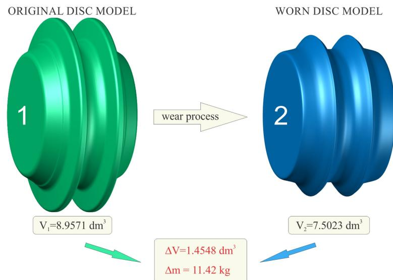
**Figure 16.** A 3D model of an original (No. 1) disc cutter and a worn (No. 2) double disc cutter created based on the original and worn profiles with calculated volume and mass losses due to wear.
