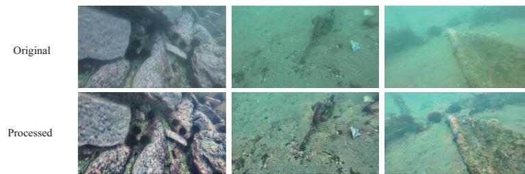
Figure 2. Comparison of underwater images before and after CLAHE processing.
