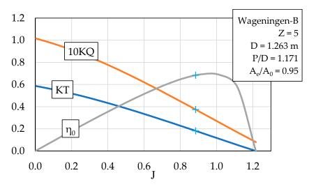
Figure 3. Propeller open-water diagram of the selected propeller.
