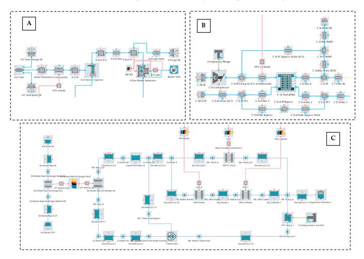
**Figure 5.** Block diagrams of the PEM subsystems: (**A**) anode subsystem, (**B**) cathode subsystem, and (**C**) thermal management subsystem.
