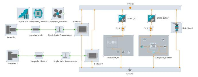
Figure 2. Block diagram of the full-electric powertrain for the catamaran demi-hull.
