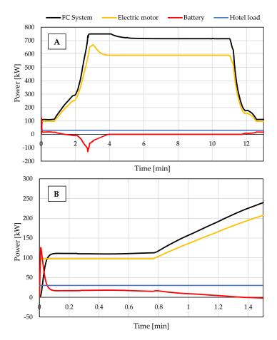
**Figure 8.** (**A**) Power variation over the routing profile for the electric motor, hotel load, fuel cell, and battery; (**B**) details of the battery and fuel cell systems' behaviors during the start-up phase.
