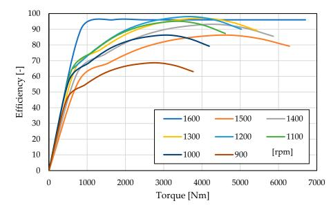
Figure 4. Electric motor efficiency-torque characteristic curves as a function of the rotation speed.
