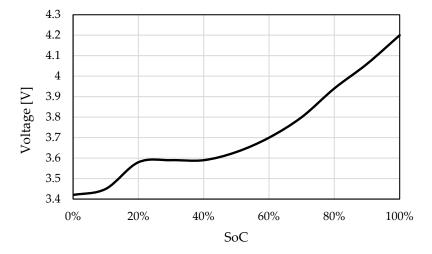
Figure 6. Open-circuit voltage and ohmic resistance variations as a function of the SoC.
