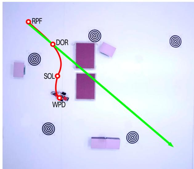
**Figure 12.** Simulation at the robotic test bed. The fault event  $eER$  led to *WPD* state, and a collision with the obstacle was avoided.
