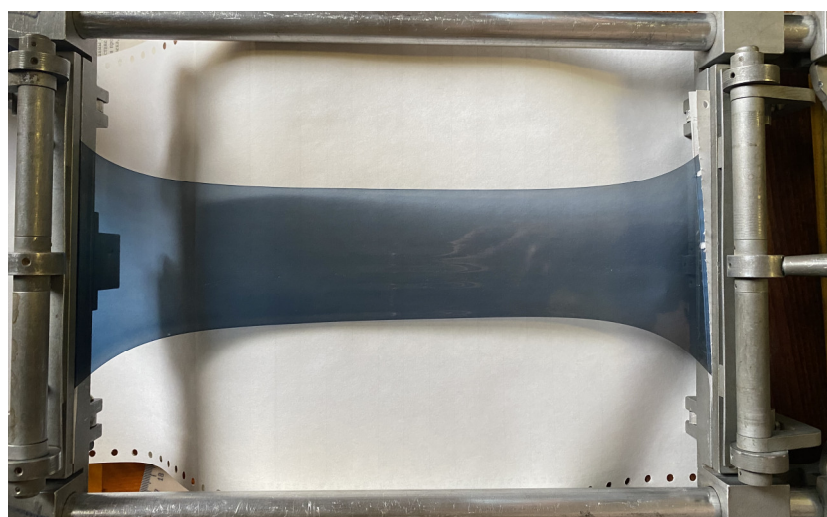
Figure 1. General view of the synthesized polarizing film in a stretchable frame.
