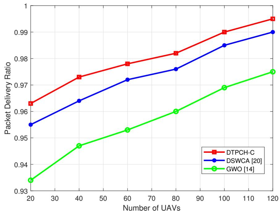
**Figure 11.** Packet delivery ratio of different clustering schemes with varying numbers of UAV nodes.
