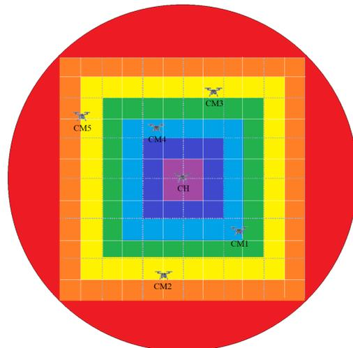
**Figure 3.** Each color grid represents the power required by the cluster head to transmit the signal. The transmitting power corresponding to different grids is shown in Table 2. (Note that this figure is a demonstration diagram for easy narration, the specific range is adjusted according to the calculation).
