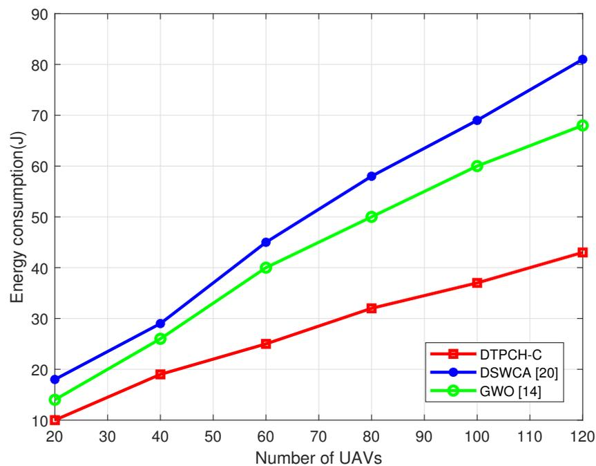
Figure 9. Energy consumption of different clustering schemes versus the number of UAV nodes.
