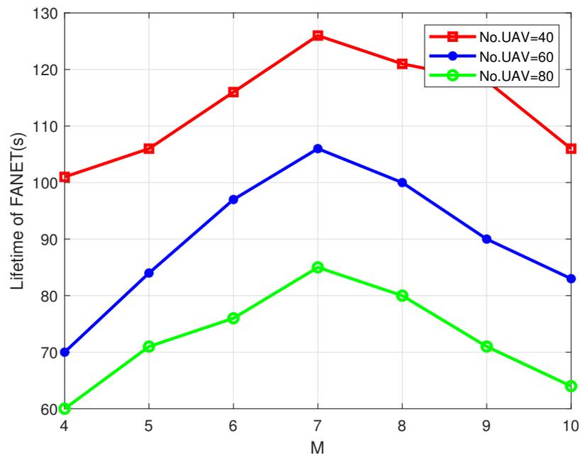
Figure 8. Lifetime of FANET in different numbers of UAV nodes versus the number of intervals M.
