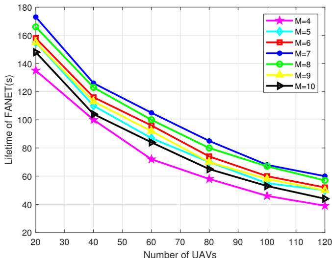
Figure 7. Lifetime of FANET in different grid partitioning conditions versus the number of UAV nodes.
