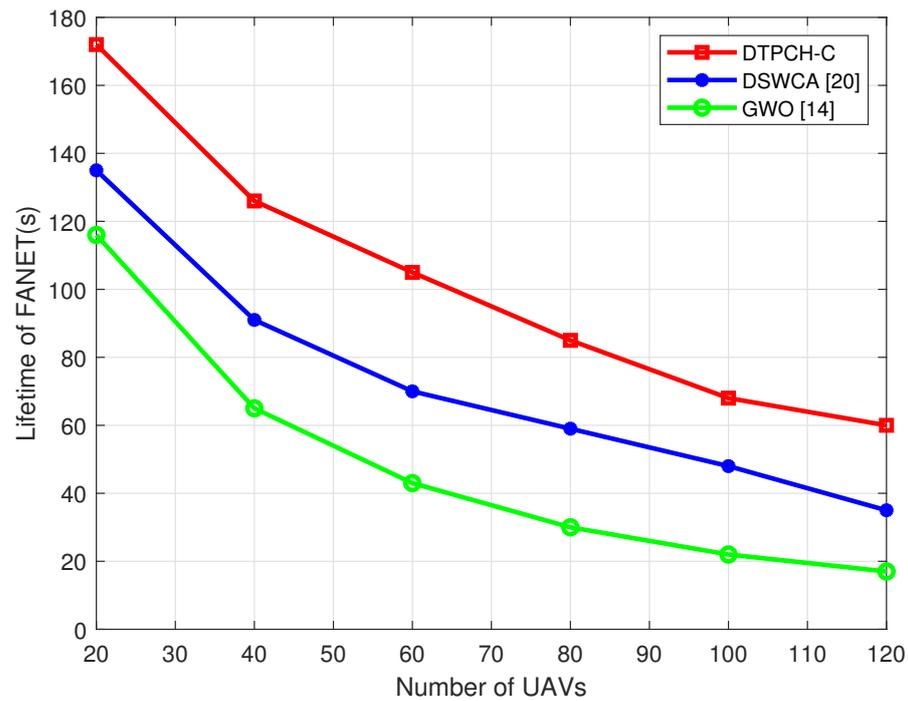
**Figure 10.** Lifetime of FANET in different clustering schemes versus the number of UAV nodes.
