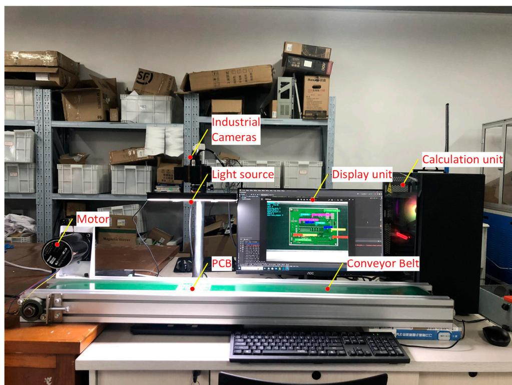
**Figure 4.** PCB surface defects real-time detection experimental platform.
