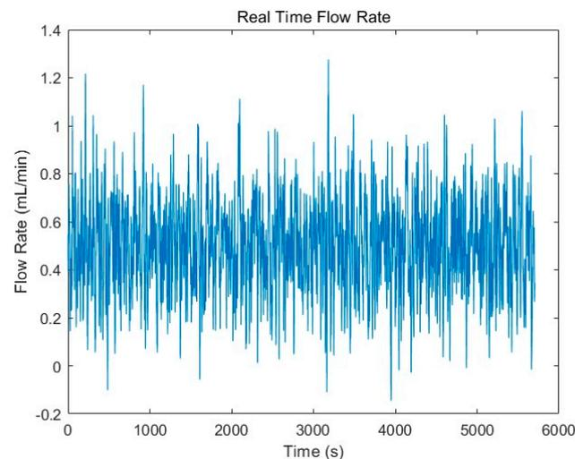
**Figure 16.** 0.5 mL/min actual flow rate reading.
