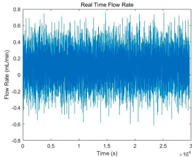
**Figure 15.** 0.1 mL/min actual flow rate reading.
