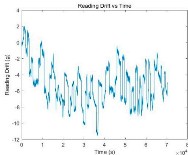
**Figure 7.** Reading drift vs. time with scale factor calibration.
