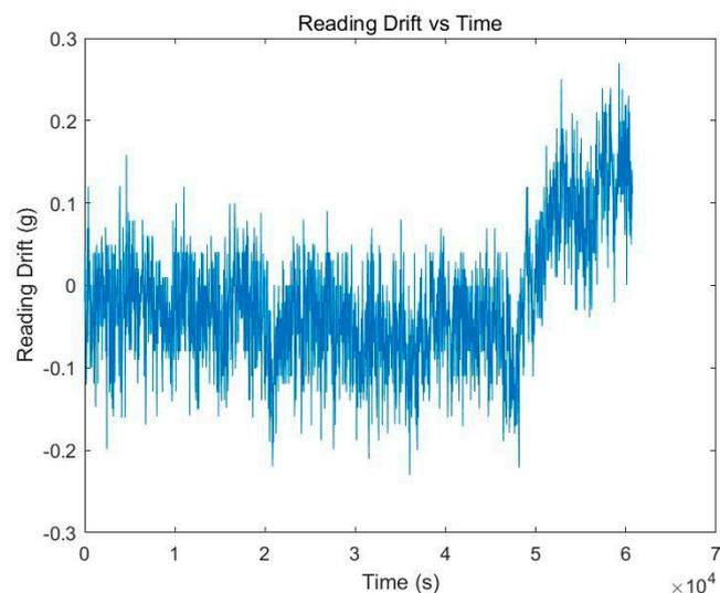
Figure 6. Drift vs. time with offset calibration.
