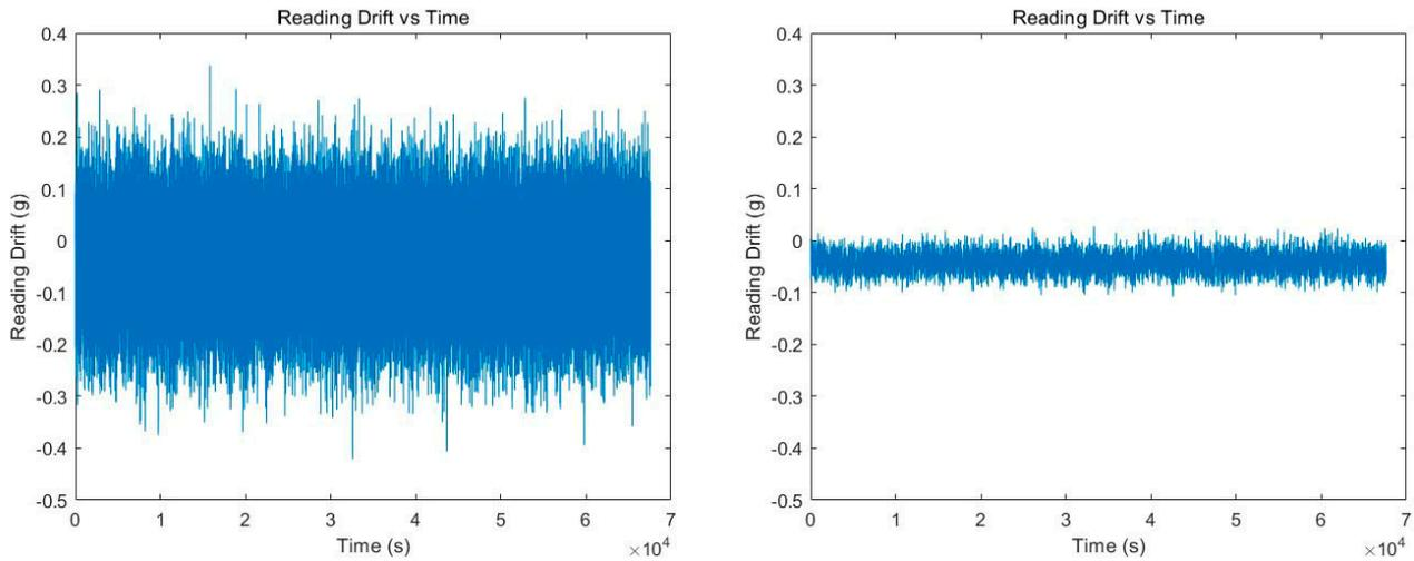
Figure 13. Unfiltered (Left) and filtered (Right) reading drift with no load.
