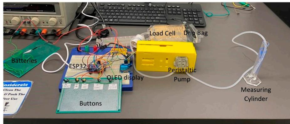
**Figure 18.** Overall measurement setup for weight sensor feedback.
