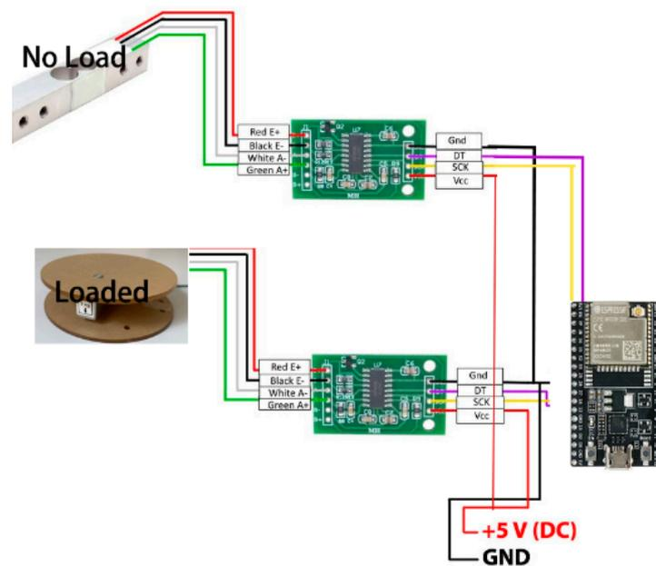
Figure 5. Offset calibration setup.
