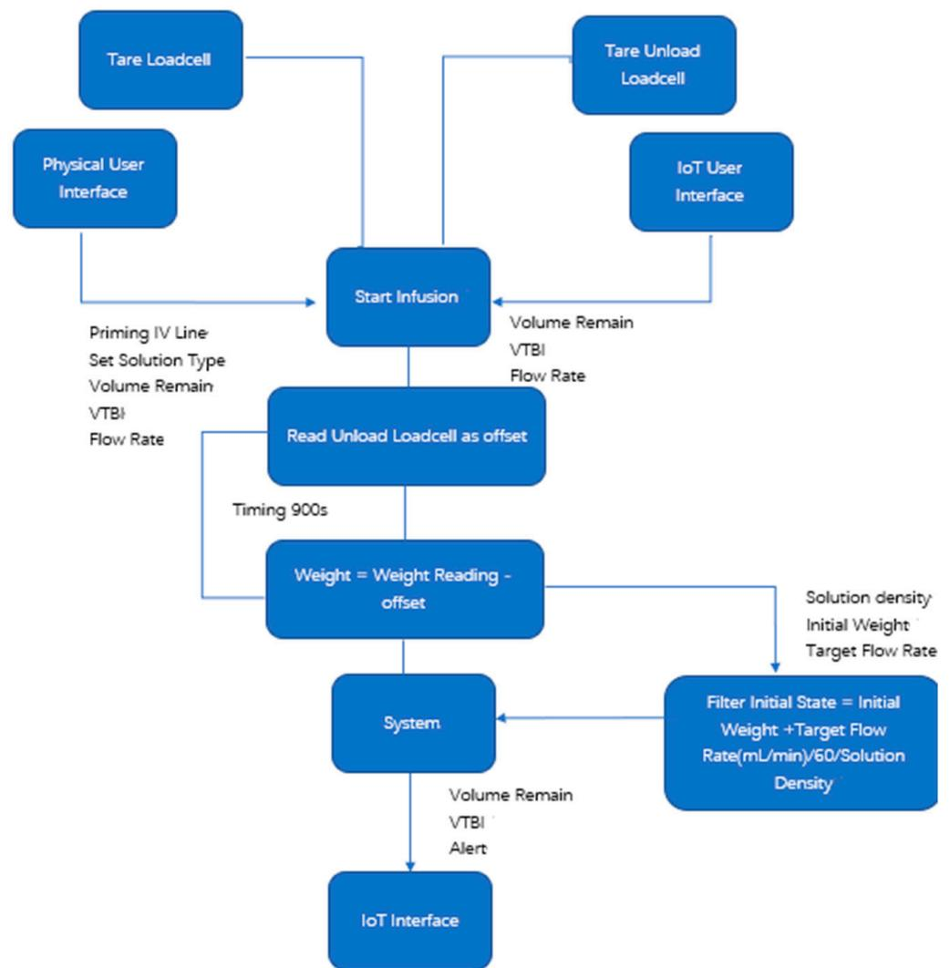
Figure 11. Block diagram of calibration process and integration with IoT.
