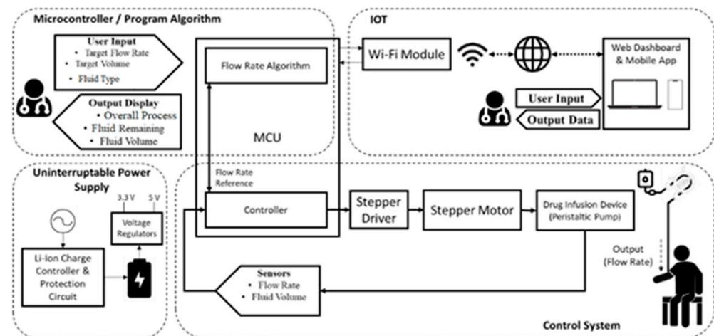
**Figure 1.** Overall block diagram of the project [26].
