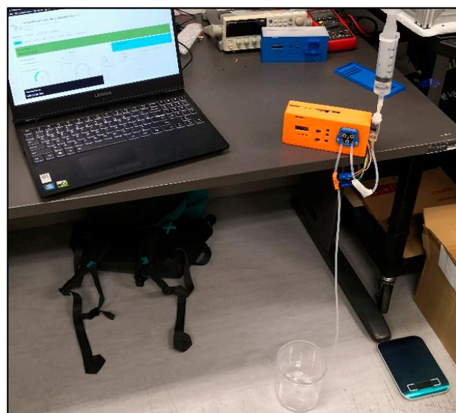
**Figure 19.** Overall measurement setup for opposed laser photoelectric sensor feedback.
