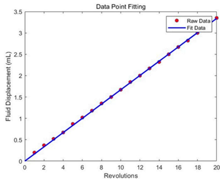
Figure 10. Fluid displacement per revolution fitting result.
