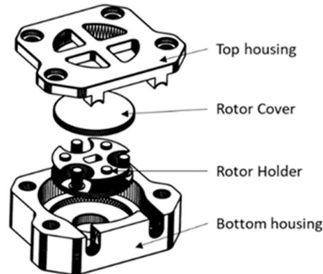
Figure 9. CAD model for the peristaltic pump.
