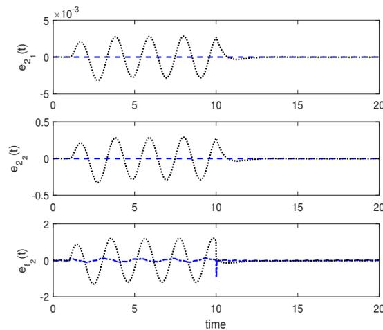
**Figure 8.** Results of the estimated error of the second subsystem: Theorem 1 (dashed) and Corollary 1 (dotted).
