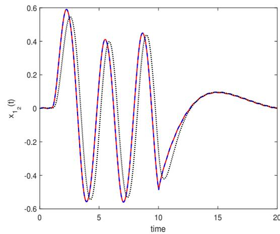
**Figure 2.** Results of the second state for the first subsystem:  $x_{1_2}(t)$  (solid),  $\hat{x}_{1_2}(t)$  from Theorem 1 (dashed) and  $\hat{x}_{1_2}(t)$  from Corollary 1 (dotted).
